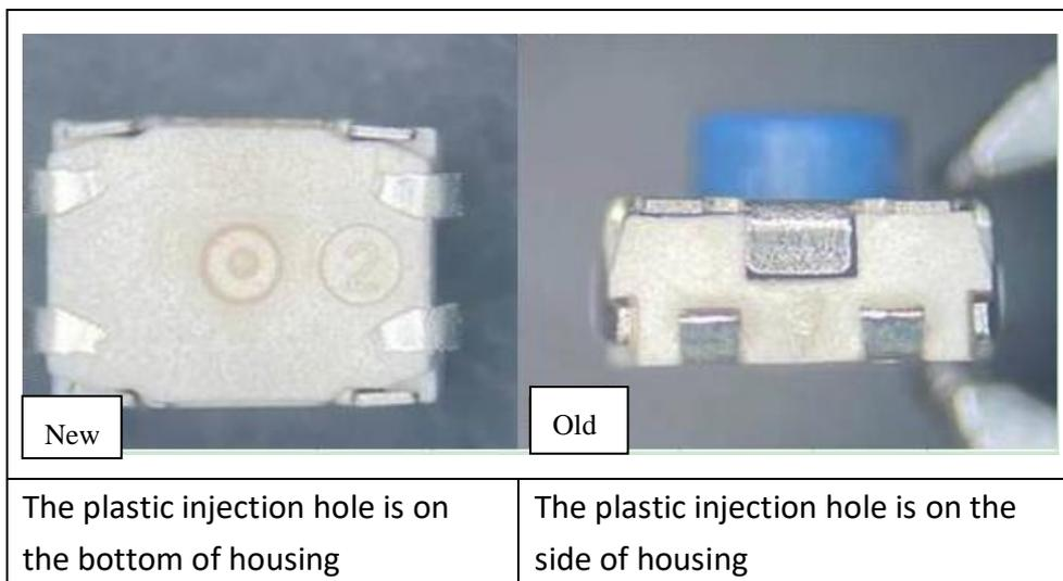
**Figure 1:** Housing injection molding location change
