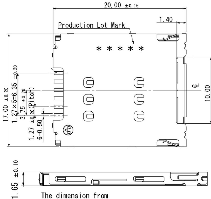
The dimension from the bottom of solder terminal to the top of the connector.
