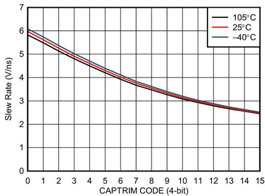
**Figure 9-2. Output Slew Rate vs. CAPTRIM Code**
