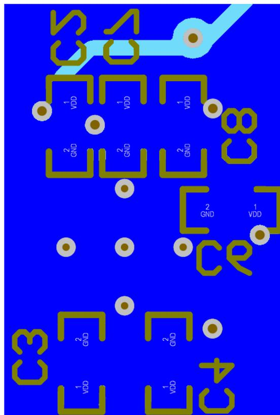
Figure 11-3. PCB Layout Example for CDCDB400, Bottom Layer
