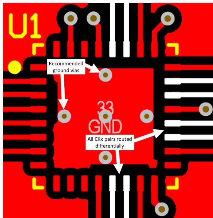
Figure 11-1. PCB Layout Example for CDCDB400, Top layer
