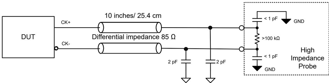
Figure 7-1. AC Test Load (Referencing Intel DB2000QL Document)
