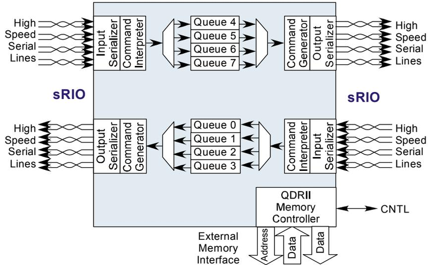
Figure 5. SerB as a FIFO between two FPGAs
