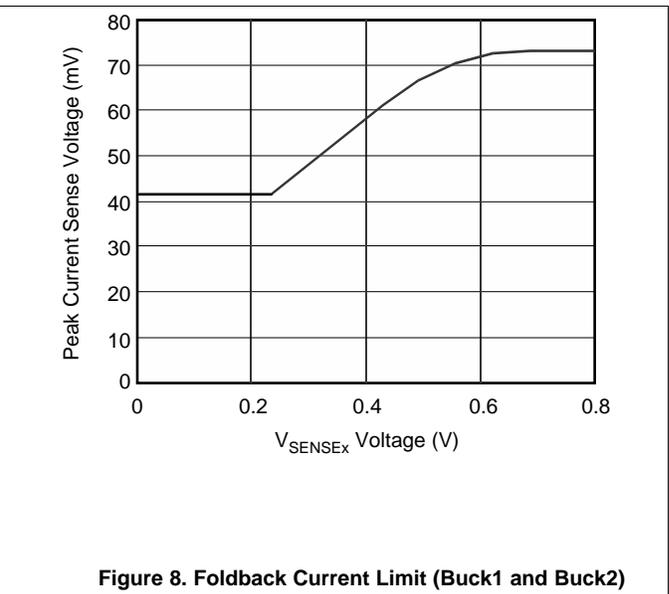
Figure 8. Foldback Current Limit (Buck1 and Buck2)
