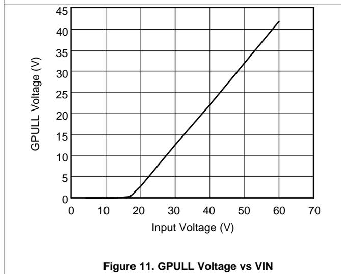
Figure 11. GPULL Voltage vs VIN
