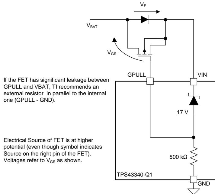
If the FET has significant leakage between GPULL and V<sub>BAT</sub>, TI recommends an external resistor in parallel to the internal one (GPULL - GND).
