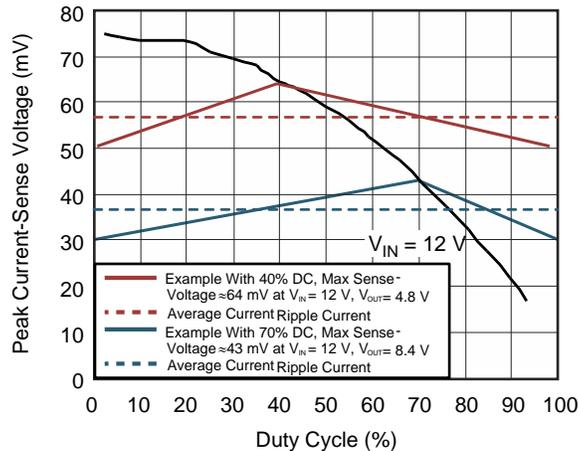
Figure 18. Peak Current-Sense Voltage versus Duty Cycle
