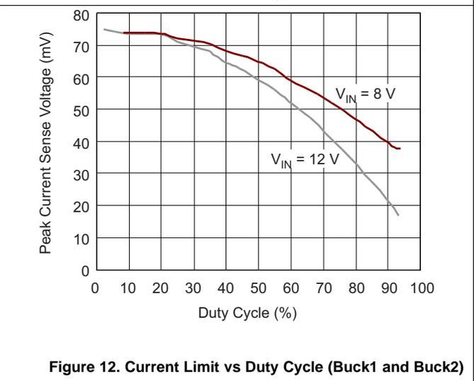
Figure 12. Current Limit vs Duty Cycle (Buck1 and Buck2)
