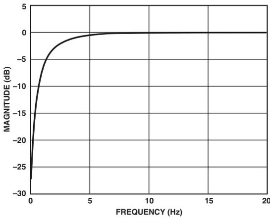
TPC 2. ADC High-Pass Filter Response,  $f_s = 48$  kHz
