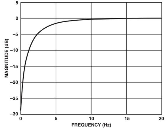
TPC 4. ADC High-Pass Filter Response,  $f_s = 96$  kHz
