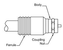
3) Crimp the ferrule using the correct tool for the connector.
