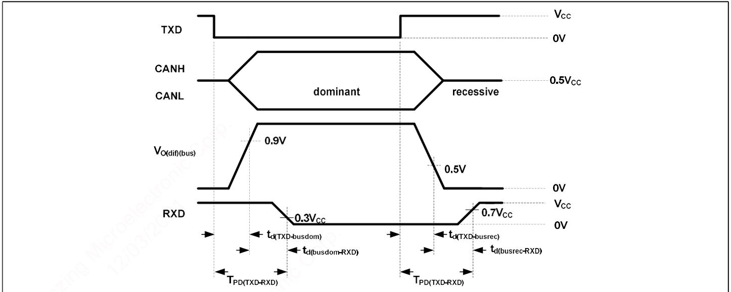
Figure 1. Timing diagram of the CAN transceiver.
