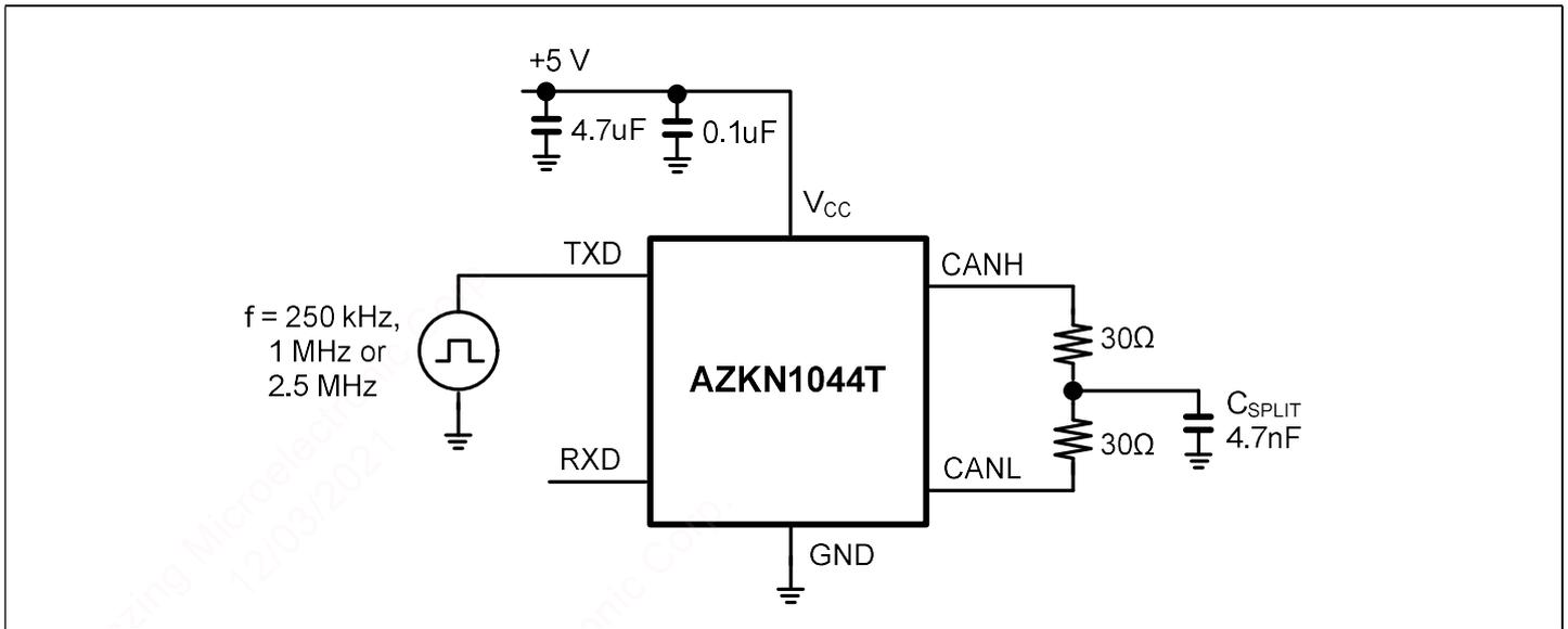
Figure 7. Test circuit for measuring transmitter driver symmetry.
