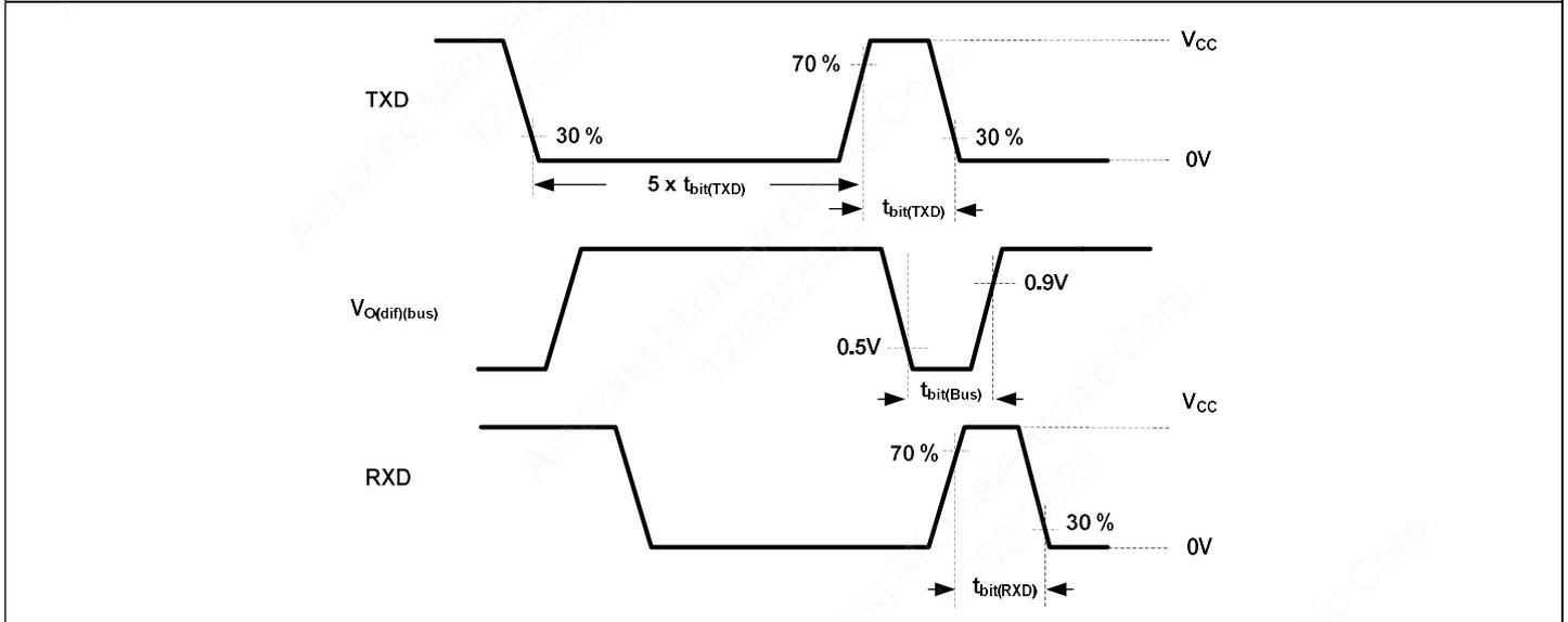
Figure 2. Timing diagram for loop delay symmetry.
