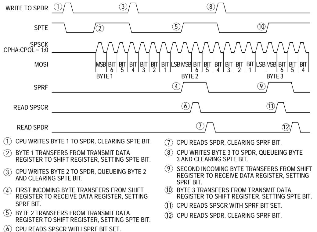
**Figure 20-8. .SPRF/SPTE CPU Interrupt Timing**
