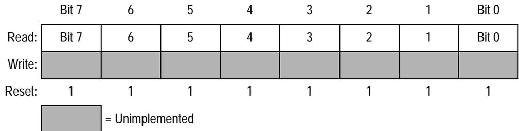
Figure 22-8. TIM Counter Modulo Register Low (TMODL)
