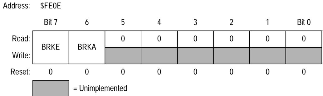
**Figure 6-3. Break Status and Control Register (BRKSCR)**
