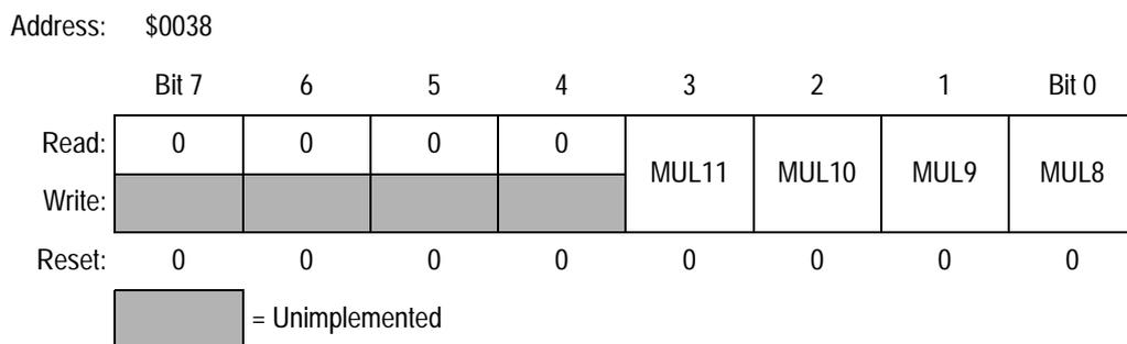
**Figure 7-6. PLL Multiplier Select Register High (PMSH)**
