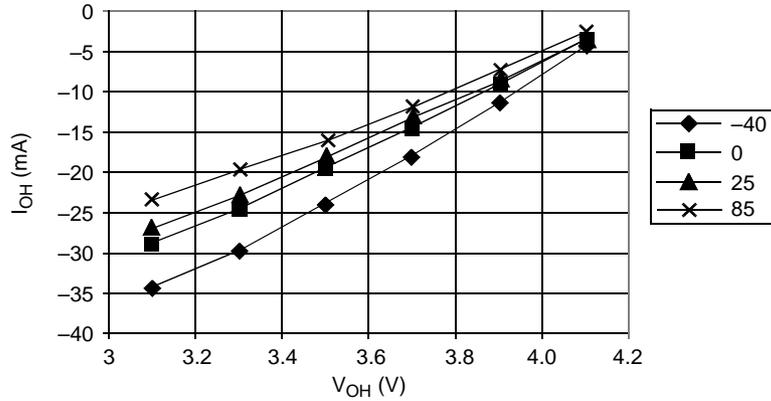
$V_{OH} > V_{DD} - 0.8 \text{ V @ } I_{OH} = -2.0 \text{ mA}$
