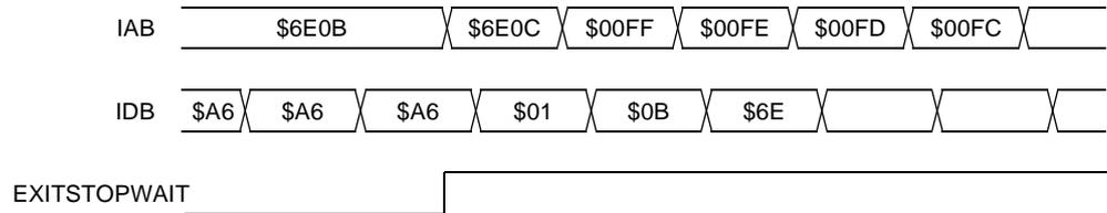
Note: EXITSTOPWAIT =  $\overline{\text{RST}}$  pin, CPU interrupt, or break interrupt
