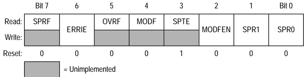
**Figure 20-14. SPI Status and Control Register (SPSCR)**
