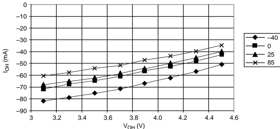
$V_{OH} > V_{DD} - 0.8 \text{ V} @ I_{OH} = -2.0 \text{ mA}$
