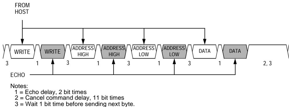
**Figure 15-6. Write Transaction**
