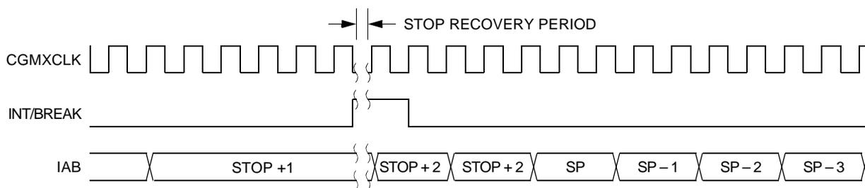
Figure 19-19. Stop Mode Recovery from Interrupt or Break
