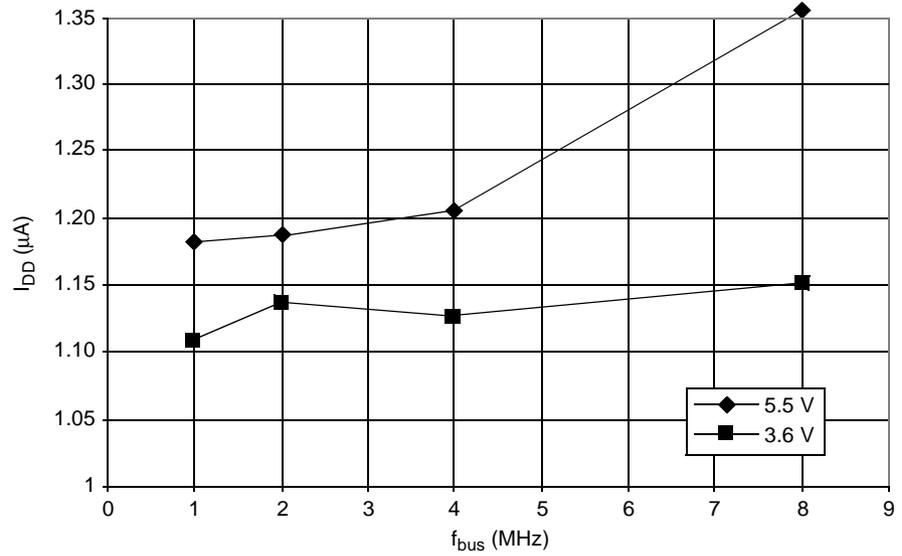
**Figure 23-15. Typical Stop Mode I<sub>DD</sub>, with all Modules Disabled
