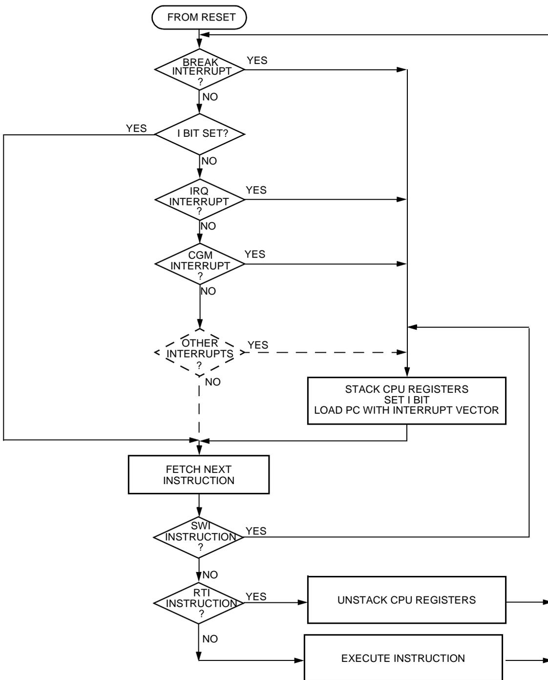
Figure 4-6. Interrupt Processing
