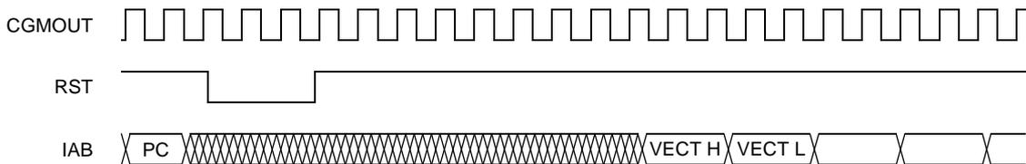
**Figure 19-4. External Reset Timing**
