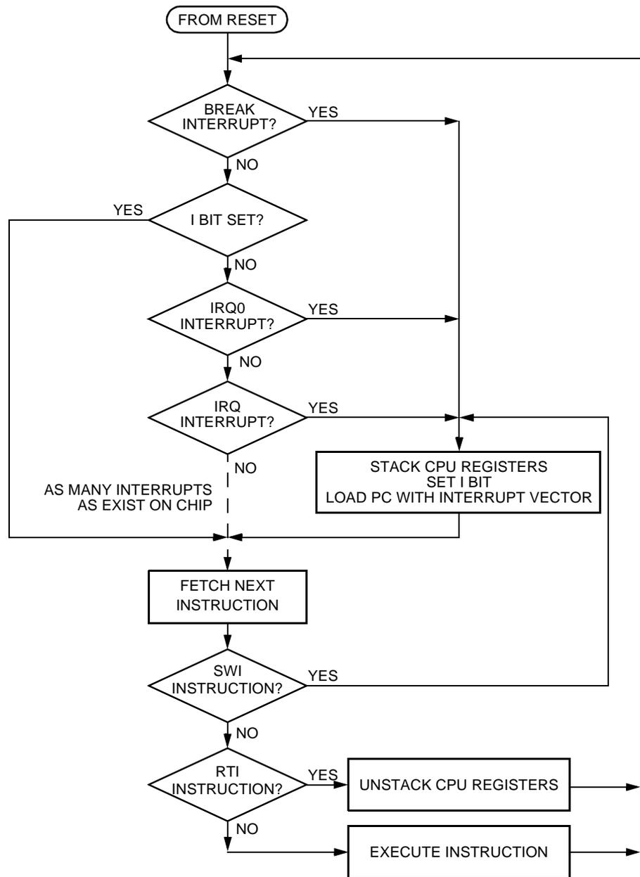
Figure 19-10. Interrupt Processing
