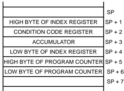
Figure 15-7. Stack Pointer at Monitor Mode Entry
