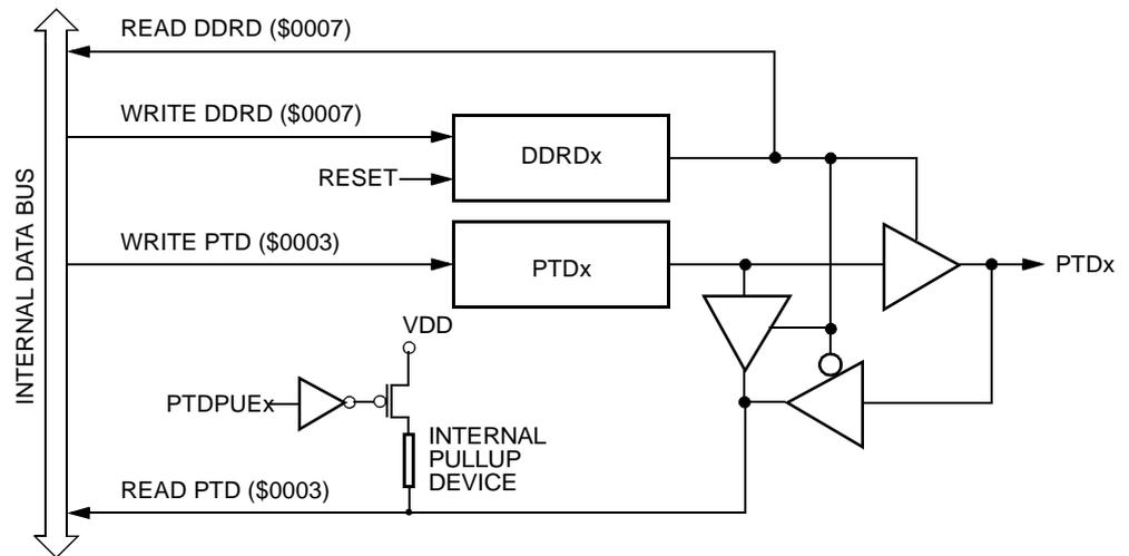
Figure 16-15. Port D I/O Circuit
