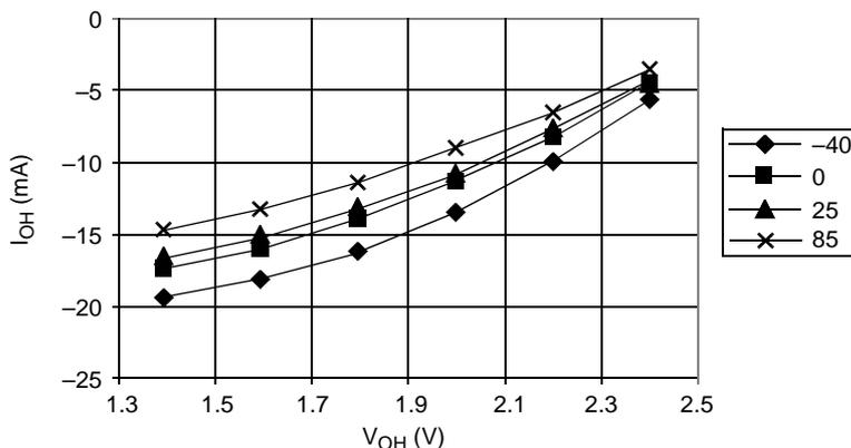
$V_{OH} > V_{DD} - 0.5\text{ V}$  @  $I_{OH} = -4.0\text{ mA}$
