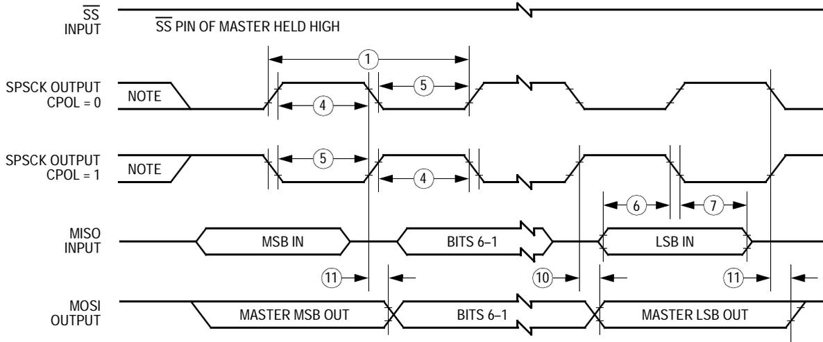
Note: This first clock edge is generated internally, but is not seen at the SPSCK pin.
