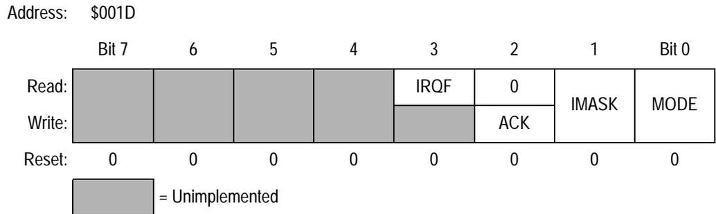
**Figure 12-3. IRQ Status and Control Register (INTSCR)**
