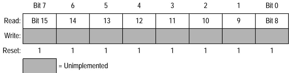
Figure 22-7. TIM Counter Modulo Register High (TMODH)
