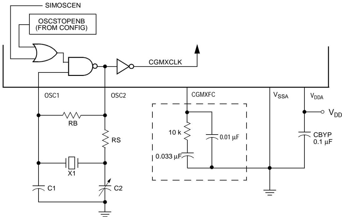
Note: Filter network in box can be replaced with a 0.47  $\mu$ F capacitor, but will degrade stability.
