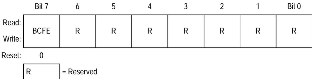
**Figure 6-7. SIM Break Flag Control Register (SBFCR)**
