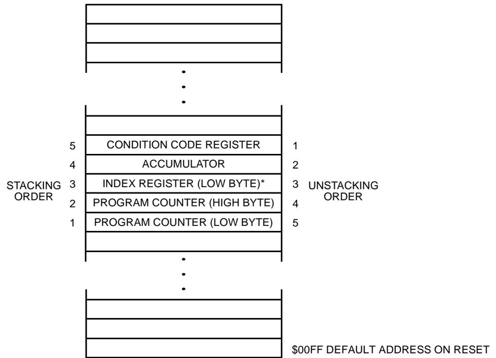
\*High byte of index register is not stacked.
