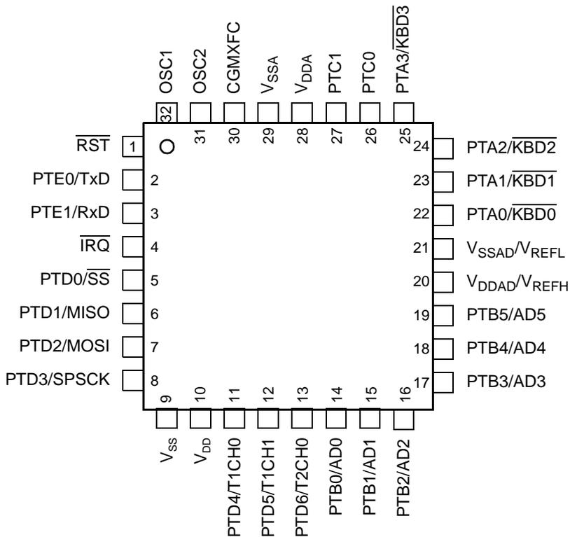
NOTE: Ports PTB4, PTB5, PTC0, and PTC1 are available only with the QFP.
