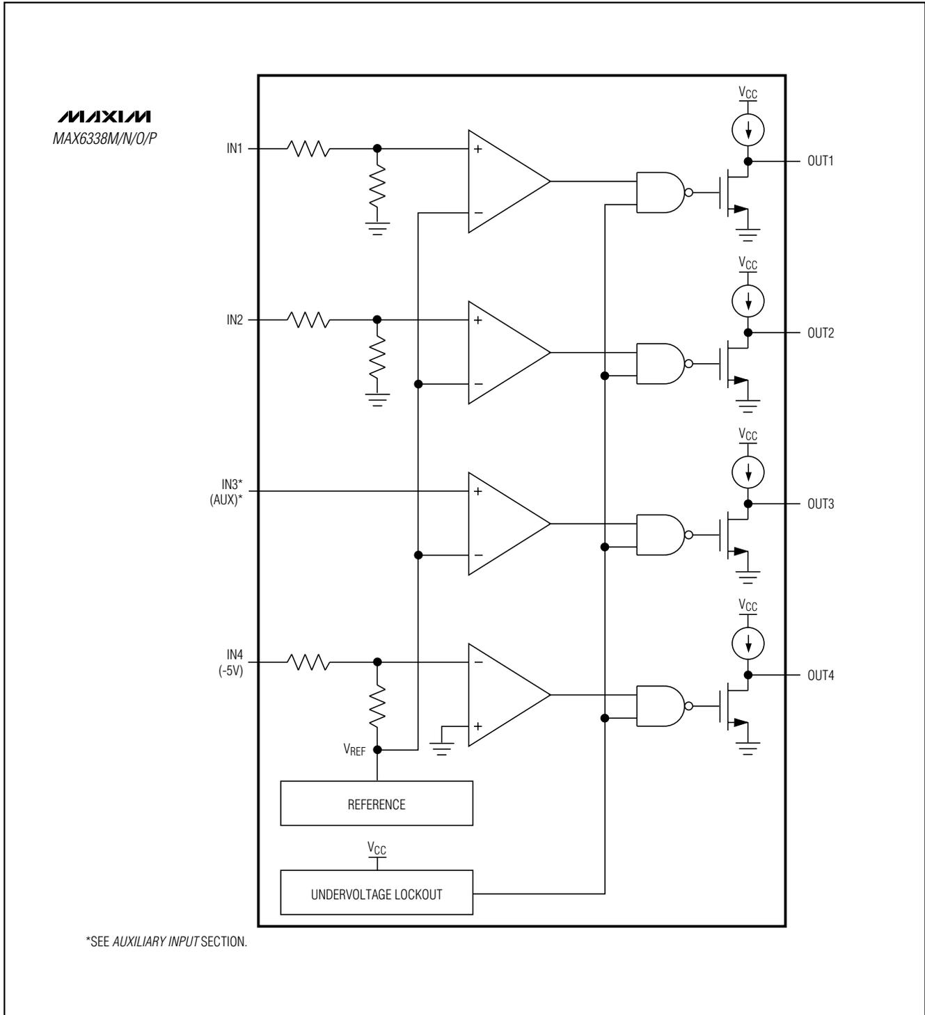
Figure 1. Functional Diagram
