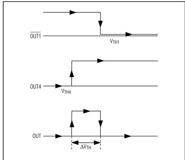
Figure 5. Output Response of Window Detector Circuit
