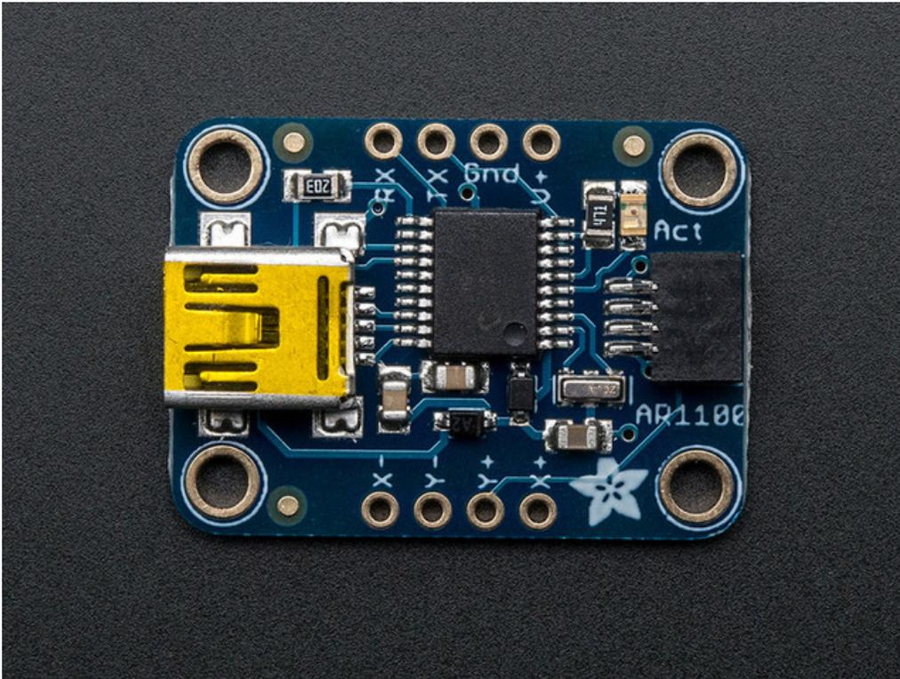
We have a breakout that features the AR1100, which has both USB and UART interfaces available. 99% of the time, you'll want to use the USB interface but there is some functionality for getting TTL UART data out (see the datasheet for details)
