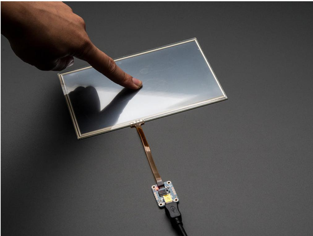
For the screens that have 1mm pitch FPC cables, you can plug the cable right into the connector. The majority of medium/large touchscreens have that kind of connector. If you have another kind of touch screen, the four X/Y
