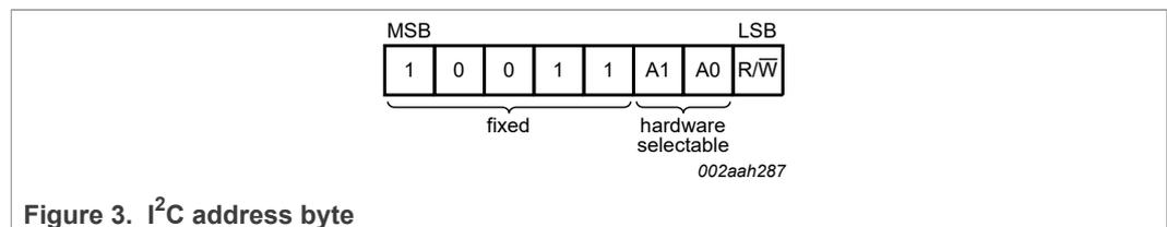
Following the address and acknowledge bit are 8 data bits which, depending on the read/write bit in the address, will read data from or write data to the non-volatile register. Data will be written to the register if the read/write bit is logic 0 and the WP input is logic 0.
