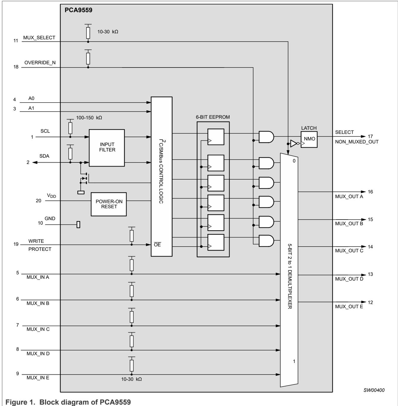
Figure 1. Block diagram of PCA9559
