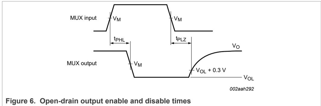
Figure 6. Open-drain output enable and disable times
