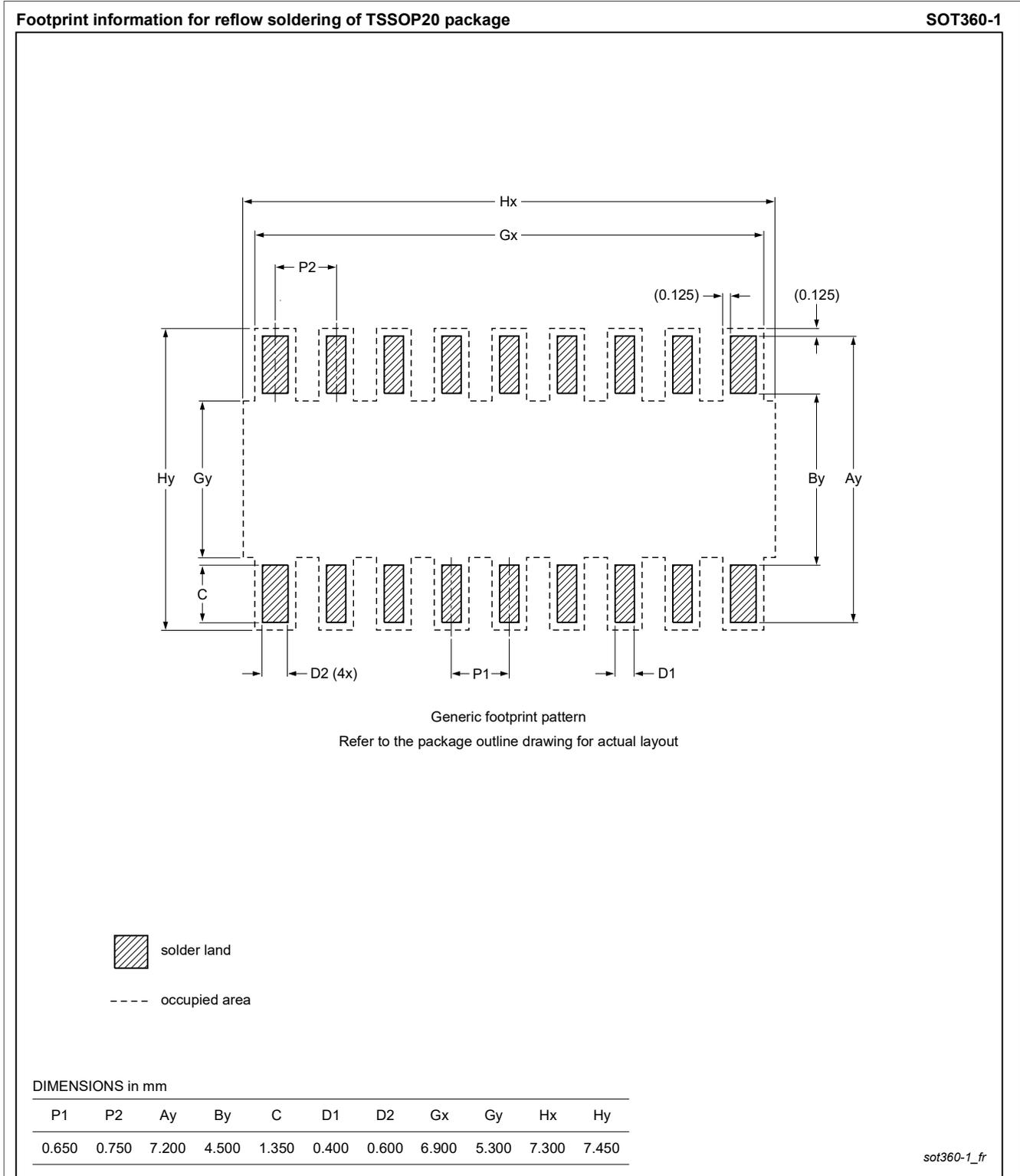
Figure 10. PCB footprint for SOT360-1 (TSSOP20); reflow soldering
