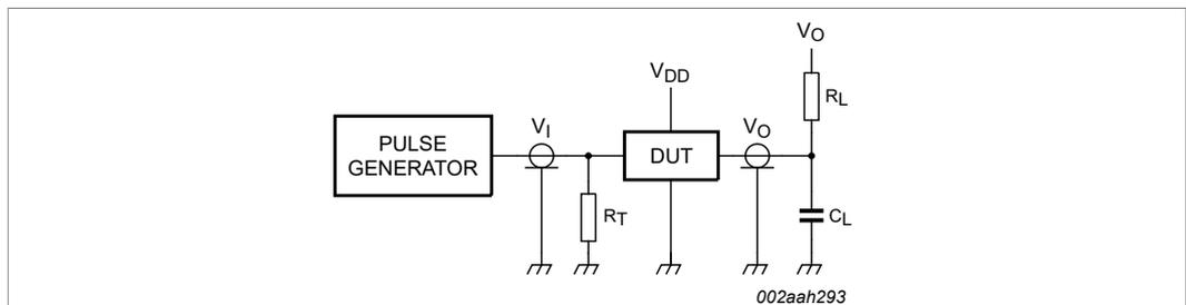
R<sub>L</sub> = load resistor; 1 kΩ.
