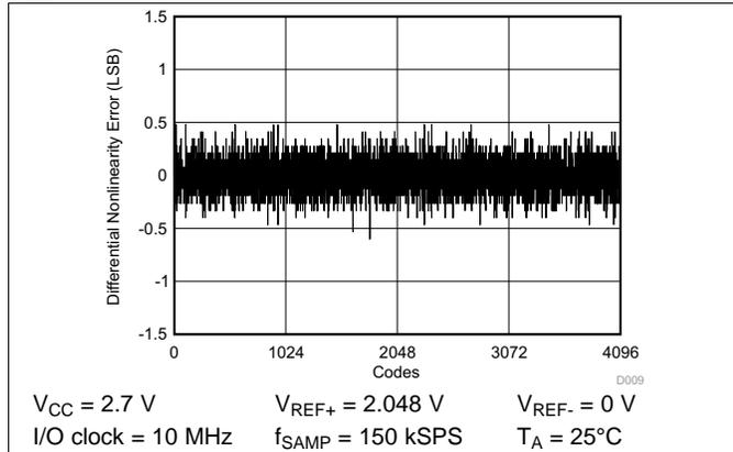
Figure 40. Differential Nonlinearity vs Digital Output Code
