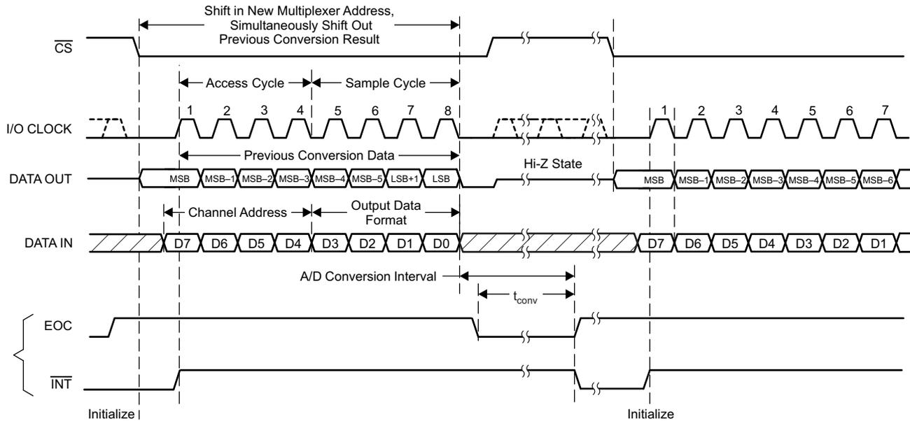
NOTE: To minimize errors caused by noise at  $\overline{CS}$ , the internal circuitry waits for a set-up time after the  $\overline{CS}$  falling edge before responding to control input signals. Therefore, no attempt should be made to clock in an address until the minimum  $\overline{CS}$  setup time has elapsed.
