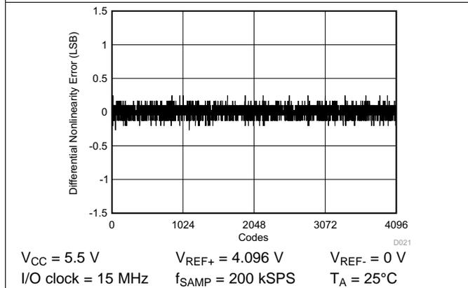
Figure 42. Differential Nonlinearity vs Digital Output Code
