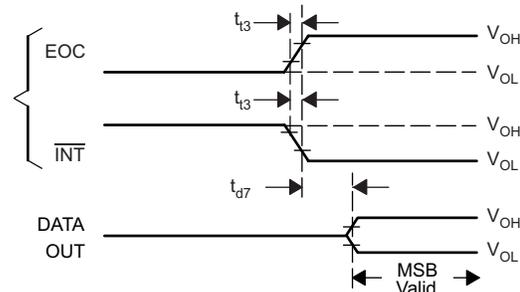
Figure 51. EOC and DATA OUT Voltage Waveforms
