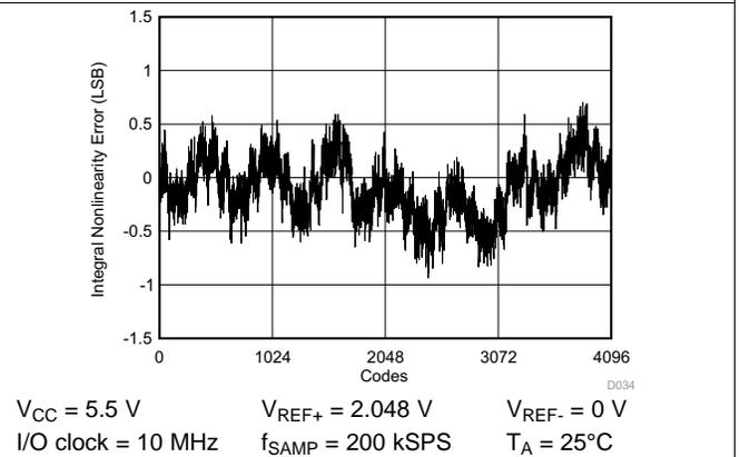
Figure 45. Integral Nonlinearity vs Digital Output Code
