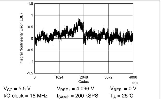
Figure 43. Integral Nonlinearity vs Digital Output Code
