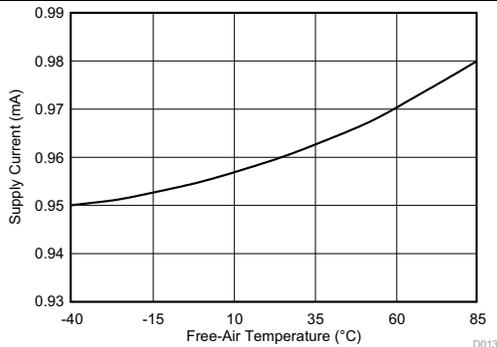
$V_{CC} = 5.5\text{ V}$        $V_{REF+} = 4.096\text{ V}$        $V_{REF-} = 0\text{ V}$
