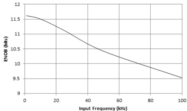
$$R_{\text{source}} = 50 \, \Omega \quad f_s = 200 \text{KSPS} \quad \text{Ext. } 4.096 \text{ V Ref.}$$
