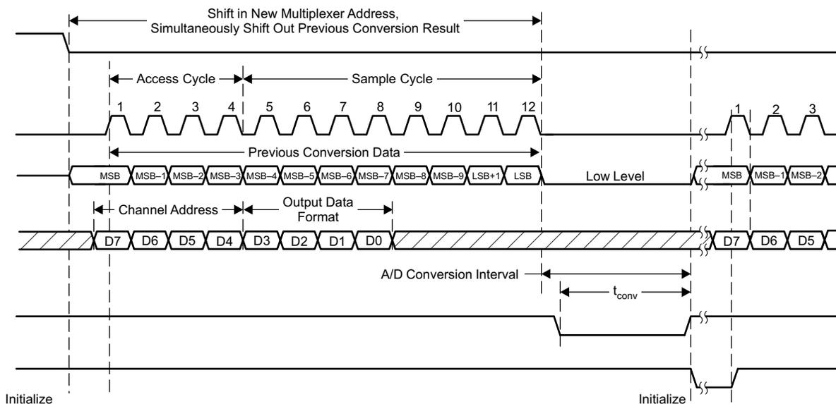
NOTE: To minimize errors caused by noise at  $\overline{\text{CS}}$ , the internal circuitry waits for a set-up time after the  $\overline{\text{CS}}$  falling edge before responding to control input signals. Therefore, no attempt should be made to clock in an address until the minimum  $\overline{\text{CS}}$  setup time has elapsed.
