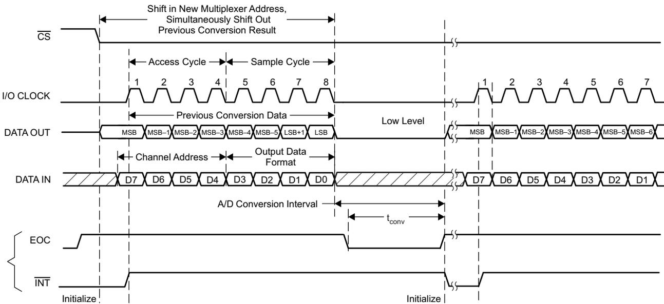
NOTE: To minimize errors caused by noise at  $\overline{CS}$ , the internal circuitry waits for a set-up time after the  $\overline{CS}$  falling edge before responding to control input signals. Therefore, no attempt should be made to clock in an address until the minimum  $\overline{CS}$  setup time has elapsed.
