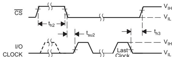
Figure 48. CS and I/O CLOCK Voltage Waveforms
