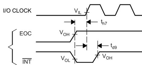
Figure 53. I/O CLOCK and EOC Voltage Waveforms
