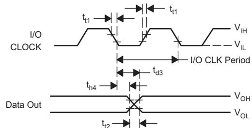
Figure 49. I/O CLOCK and DATA OUT Voltage Waveforms
