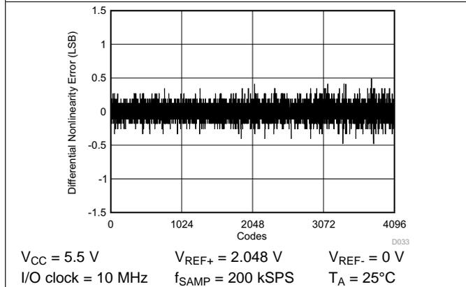
Figure 44. Differential Nonlinearity vs Digital Output Code
