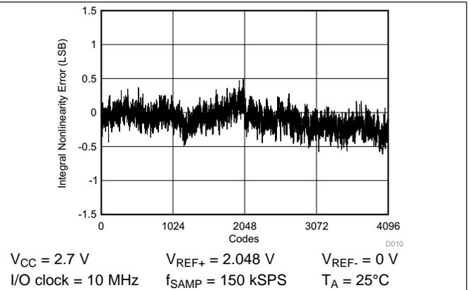
Figure 41. Integral Nonlinearity vs Digital Output Code
