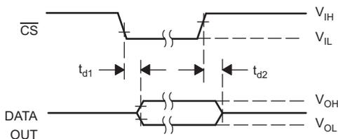
Figure 46. DATA OUT to Hi-Z Voltage Waveforms
