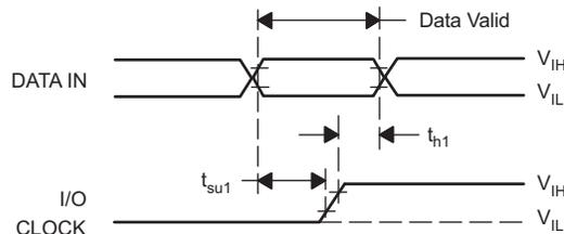
Figure 47. DATA IN and I/O CLOCK Voltage
