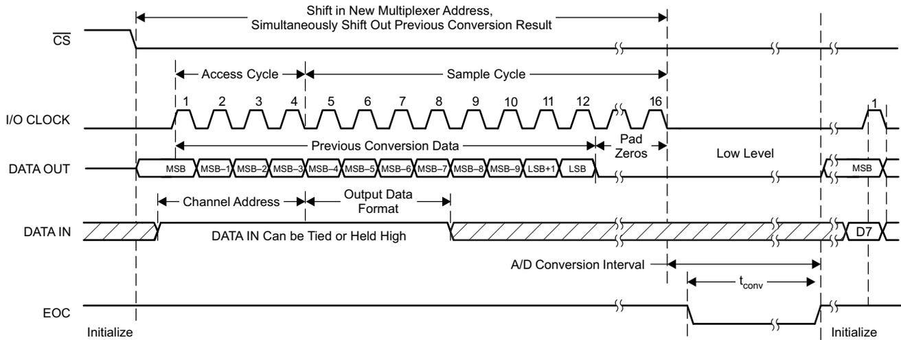
NOTE: To minimize errors caused by noise at  $\overline{CS}$ , the internal circuitry waits for a set-up time after the  $\overline{CS}$  falling edge before responding to control input signals. Therefore, no attempt should be made to clock in an address until the minimum  $\overline{CS}$  setup time has elapsed.
