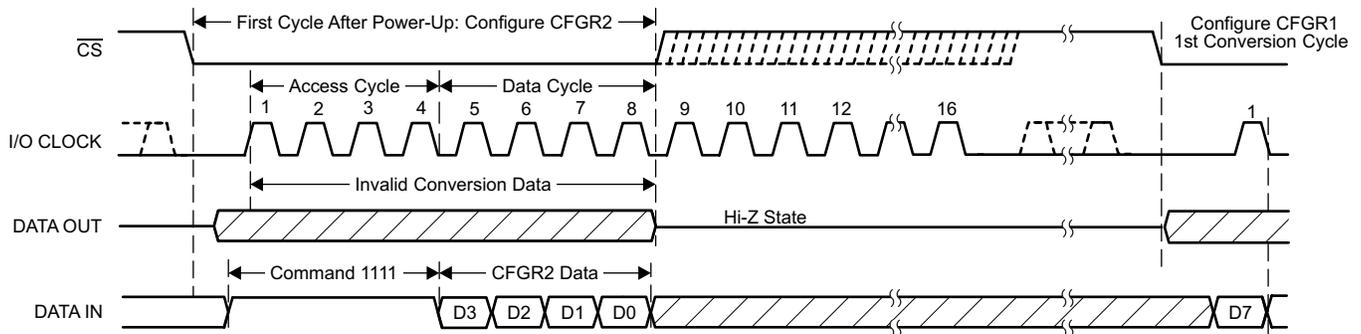
NOTE: To minimize errors caused by noise at  $\overline{\text{CS}}$ , the internal circuitry waits for a set-up time after the  $\overline{\text{CS}}$  falling edge before responding to control input signals. Therefore, no attempt should be made to clock in an address until the minimum  $\overline{\text{CS}}$  setup time has elapsed.
