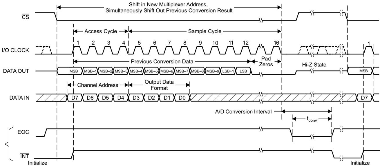
NOTE: To minimize errors caused by noise at  $\overline{CS}$ , the internal circuitry waits for a set-up time after the  $\overline{CS}$  falling edge before responding to control input signals. Therefore, no attempt should be made to clock in an address until the minimum  $\overline{CS}$  setup time has elapsed.
