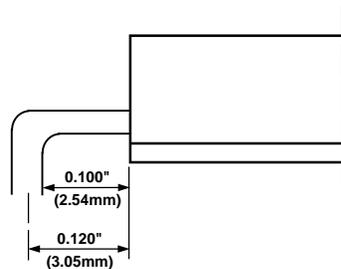
Figure 27. Minimum Bend Radius of 40 Mil (1.02 mm) Pins
