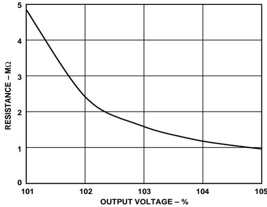
Figure 19. External Resistor Value for Increasing Output Voltage
