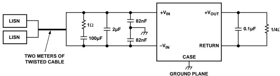
NOTE: 100μF CAPACITOR AND 1Ω RESISTOR PROVIDE STABILIZATION FOR 100μH DIFFERENTIAL SOURCE INDUCTANCE INTRODUCED BY THE LISNs. REFER TO SECTION ON EMI CONSIDERATIONS FOR MORE INFORMATION.
