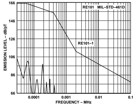
Figure 15. Radiated Emissions, MIL-STD-461D, RE101, 100 W Load
