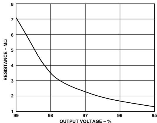
Figure 18. External Resistor Value for Reducing Output Voltage
