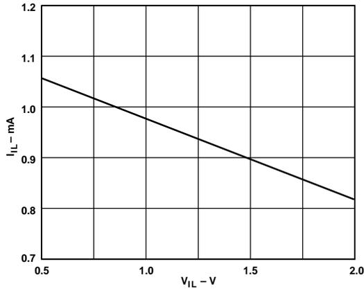
Figure 23. Input Characteristics of Pin 6 When Pulled Low
