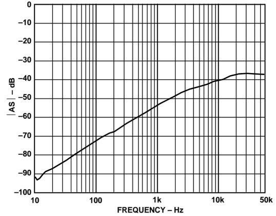
Figure 10. Audio Susceptibility (Magnitude of  $V_{OUT}/V_{IN}$ )
