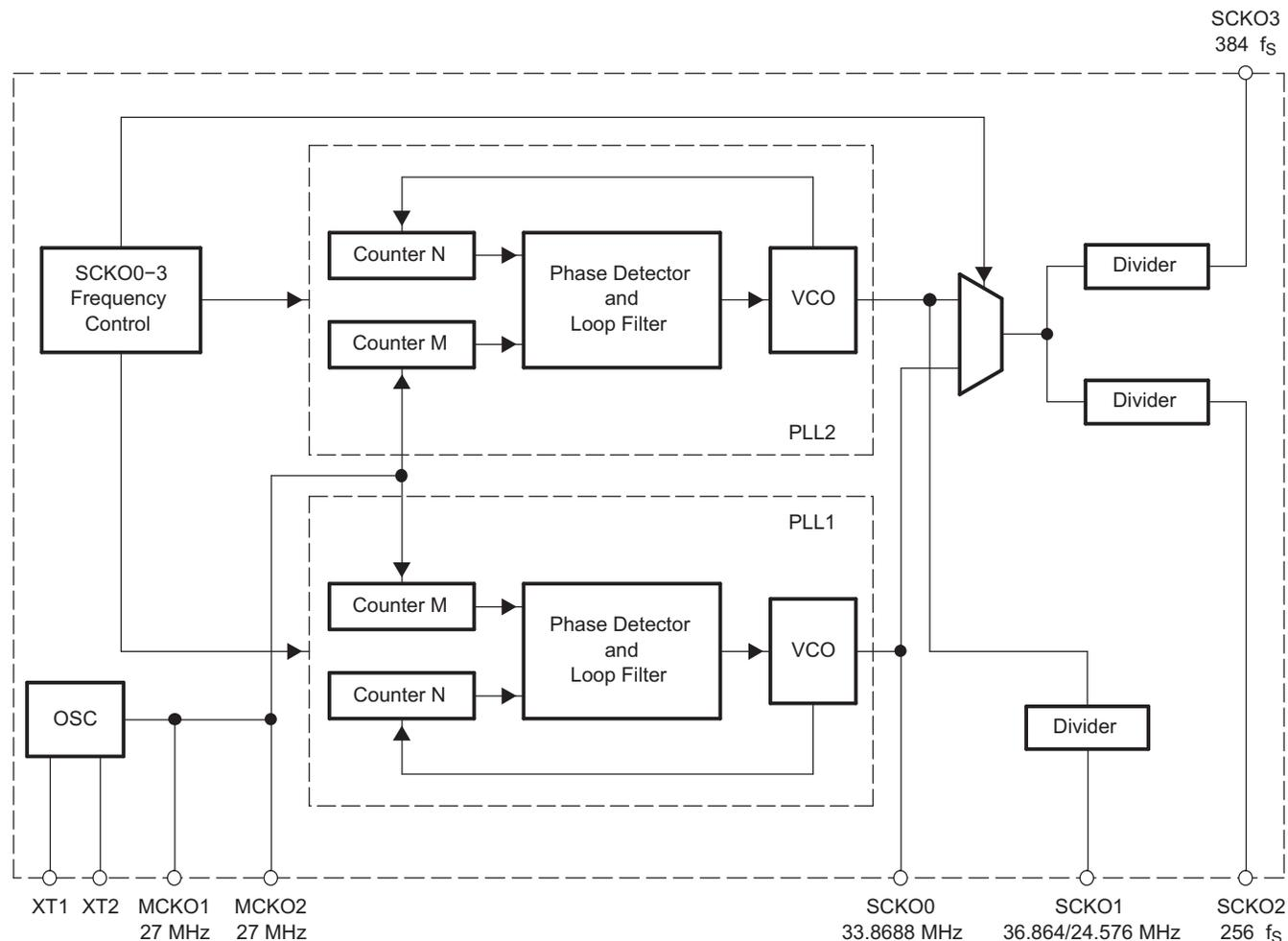
Figure 7. Block Diagram
