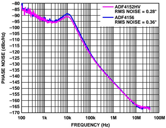
Figure 6. Active Filter Phase Noise, ADF4152HV vs. ADF4156; Active Filter Implemented Using OP27 Op Amp; PFD = 20 MHz, Loop Bandwidth = 10 kHz,  $I_{CP} = 300 \mu A$ , Carrier Frequency = 1.7 GHz,  $V_P = 28 V$
