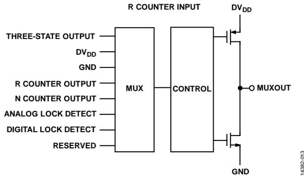
Figure 18. MUXOUT Schematic
