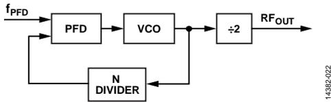
Figure 27. PLL Loop Closed Before Output Divider
