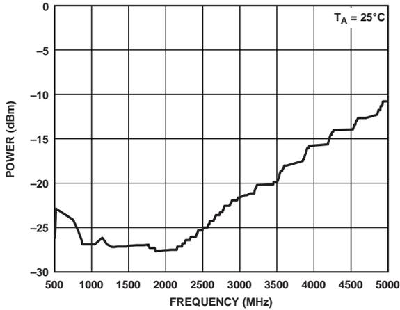
Figure 4. RF Input Sensitivity, RF Output Disabled
