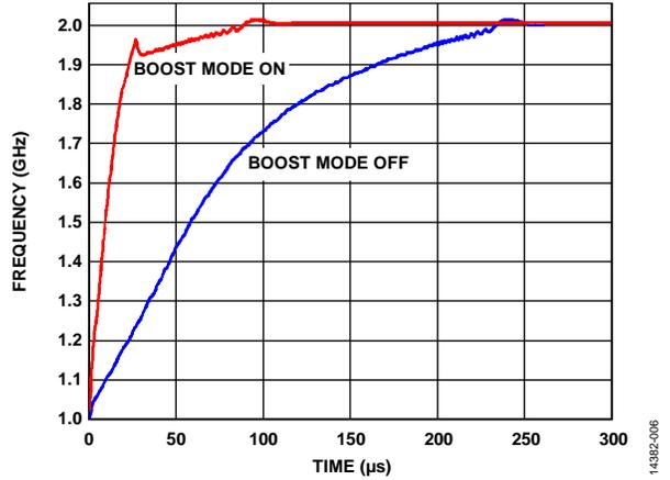
Figure 7. PLL Lock Time with Boost Mode On and Off; Locking over Octave Range Jump (1 GHz to 2 GHz) for PFD = 20 MHz, Loop Bandwidth = 100 kHz,  $I_{CP} = 300 \mu A$ ,  $V_P = 28 V$ ,  $AV_{DD} = DV_{DD} = SDV_{DD} = 3.3 V$ ,  $REF_{IN} = 100 MHz$
