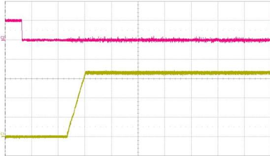
Fig. 10: Turn-on transient at full rated load current (resistive) plus 4700  $\mu$ F at  $V_{in}$  = 48 V, triggered via ON/OFF pin. Top trace: ON/OFF signal (5 V/div.). Bottom trace: output voltage(1 V/div.). Time scale: 50 ms/div.
