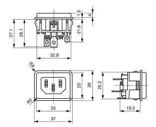
Line and neutral: Quick-connect Quick connect terminal 4.8 x 0.8 mm
