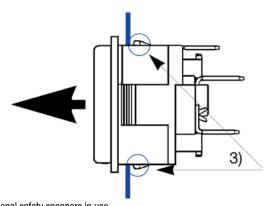
3) Additional safety snappers in use against excessive pull out force
