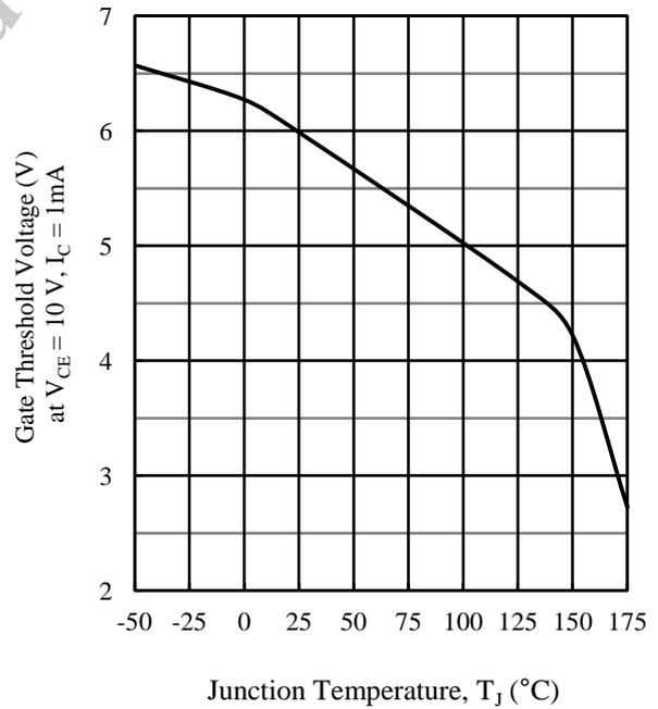
Figure 13. Gate Threshold Voltage vs. Junction Temperature
