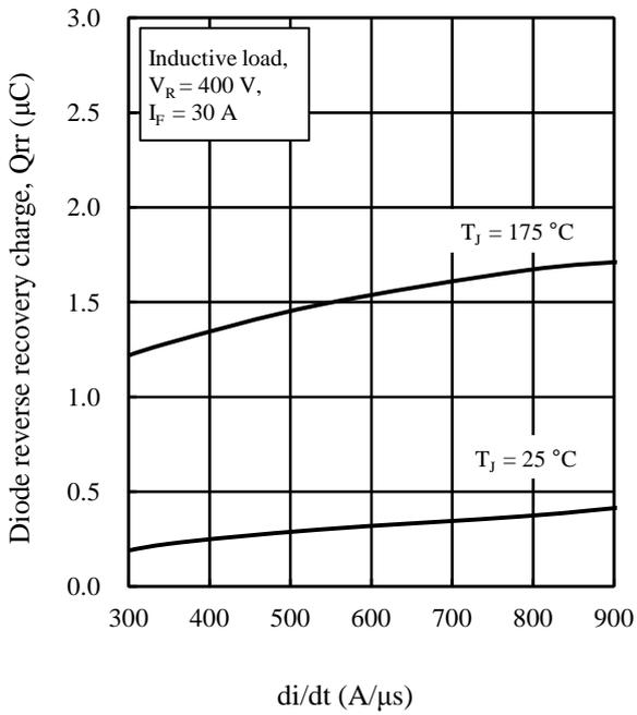
Figure 26. Diode Reverse Recovery Charge vs.  $di/dt$
