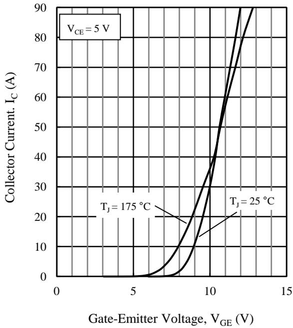
Figure 10. Transfer Characteristics
