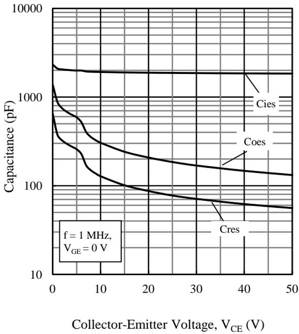
Figure 14. Capacitance Characteristics
