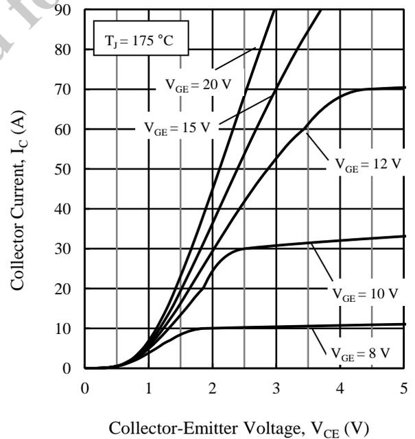
Figure 9. Output Characteristics ( $T_J = 175\text{ }^\circ\text{C}$ )
