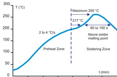
**Fig. 2. Reflow Temperature Profile for Pb-free Soldering**
