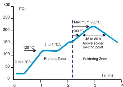
**Fig. 1. Infrared Reflow Temperature Profile for Pb-containing Soldering**
