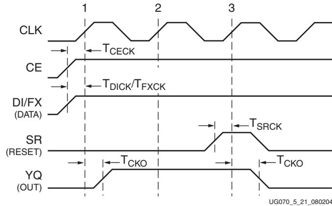
Figure 5-21: General Slice Timing Characteristics
