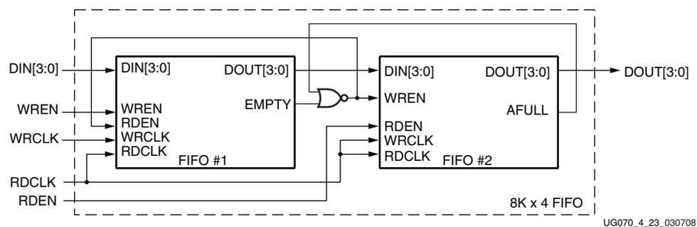
Figure 4-22: Cascading FIFO
