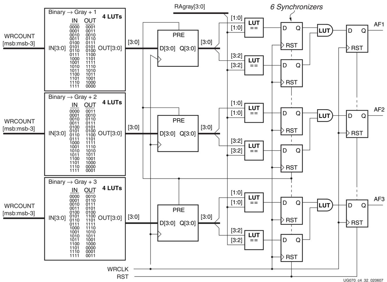
Figure 4-31: Intermediate Signal Generation for ALMOSTFULL Flag
