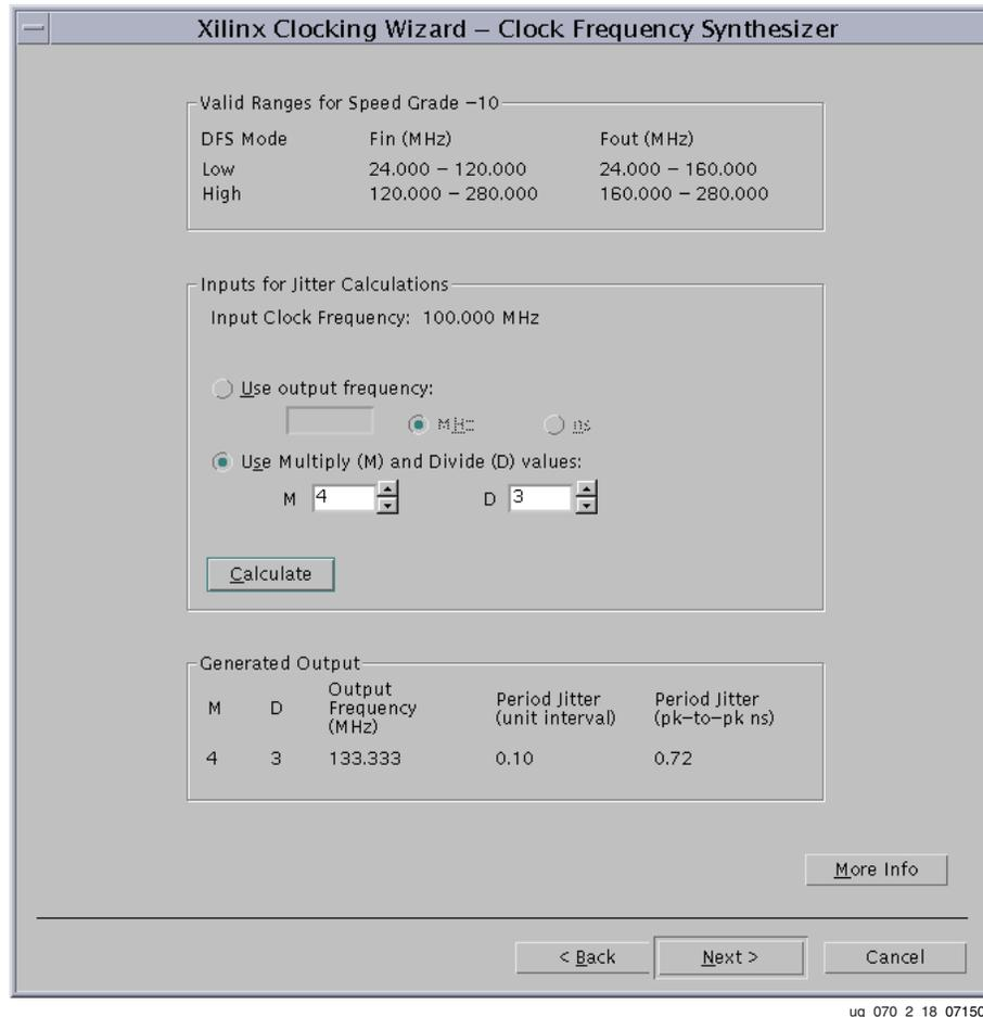
Figure 2-19: Xilinx Clocking Wizard — Frequency Synthesizer
