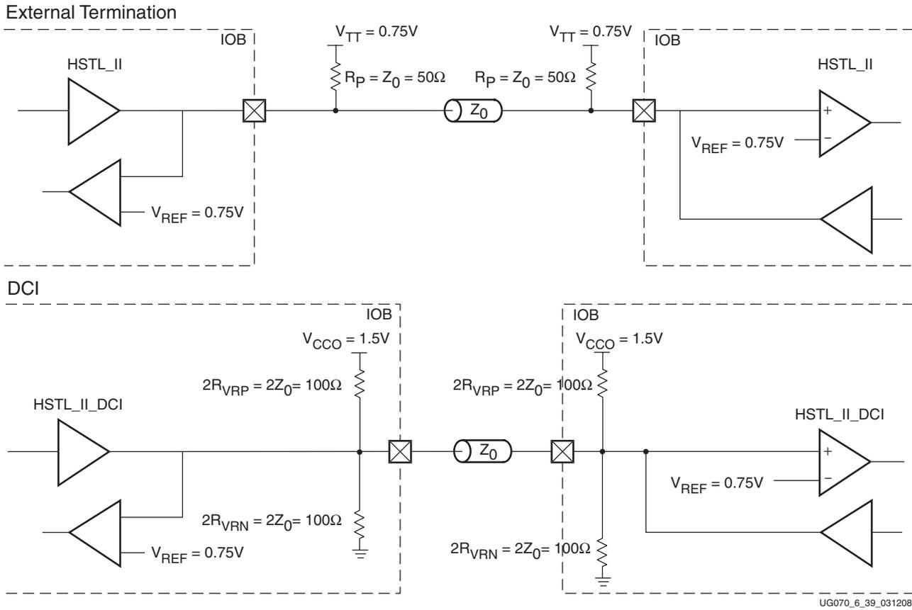
Figure 6-41: HSTL (1.5V) Class II Bidirectional Termination
