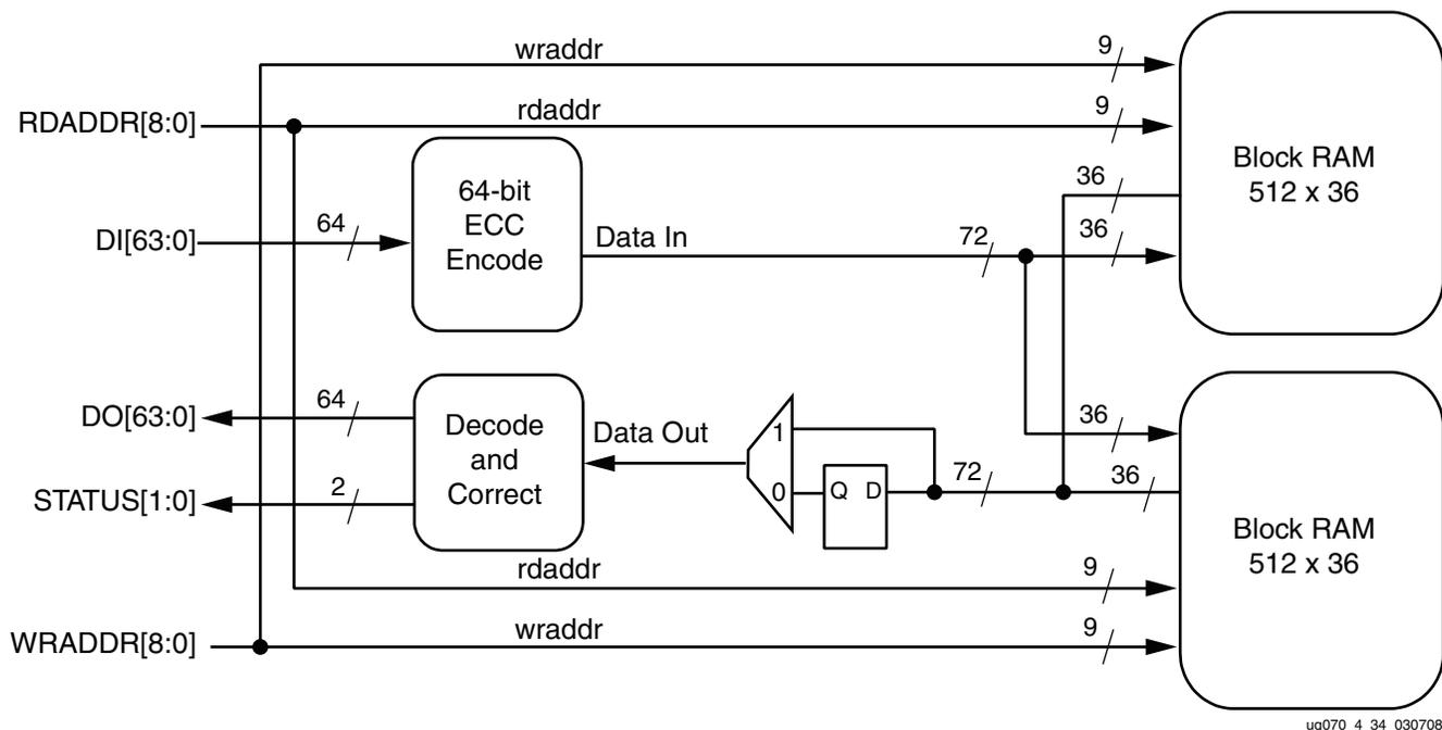
Figure 4-34: Top-Level View of Block RAM ECC
