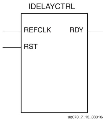
Figure 7-13: IDELAYCTRL Primitive
