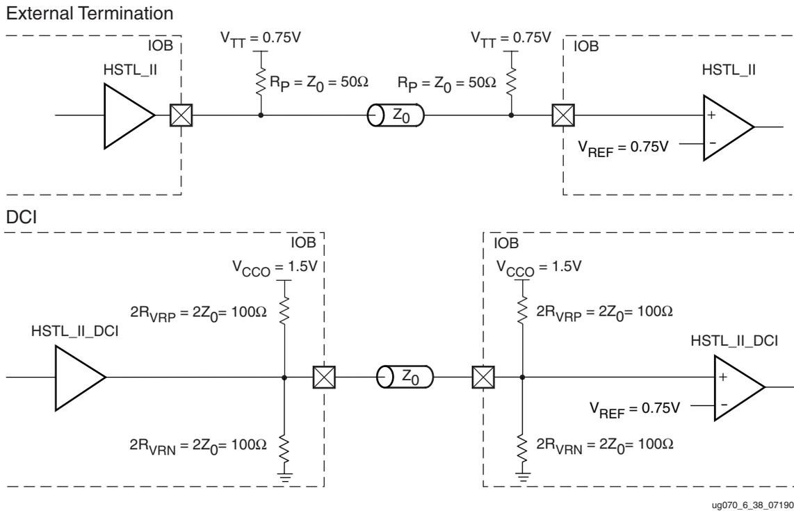
Figure 6-40: HSTL (1.5V) Class II Unidirectional Termination
