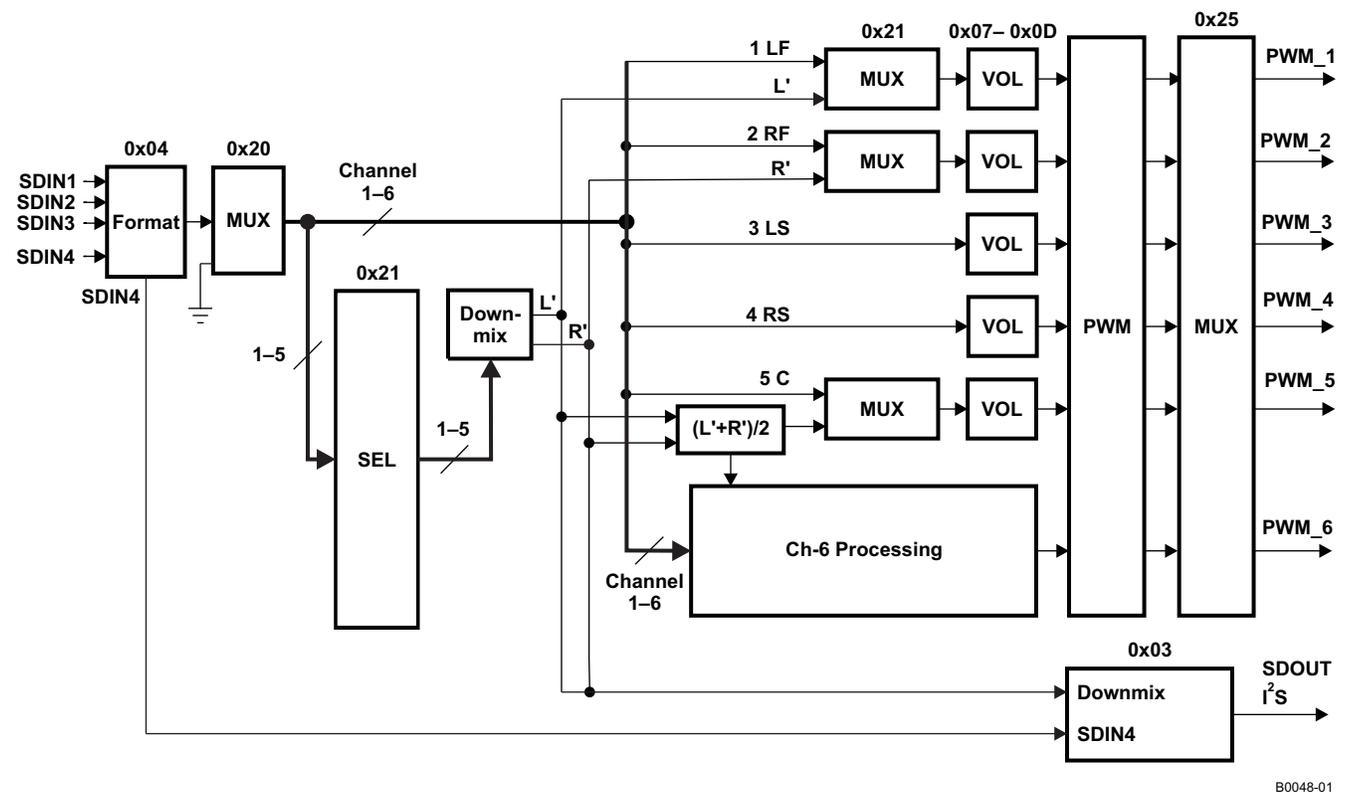
Figure 6. TAS5086 Data Flow Diagram With I<sup>2</sup>C Registers
