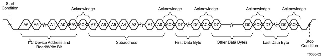
**Figure 24. Multiple-Byte Write Transfer**
