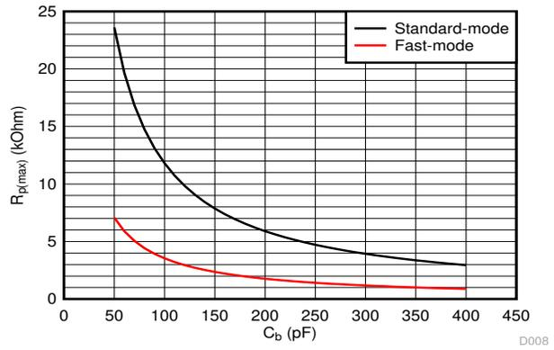
Standard-mode ( $f_{SCL} = 100$  kHz,  $t_r = 1 \mu s$ )      Fast-mode ( $f_{SCL} = 400$  kHz,  $t_r = 300$  ns)
