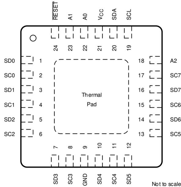
Figure 5-2. RGE Package, 24-Pin VQFN , Top View
