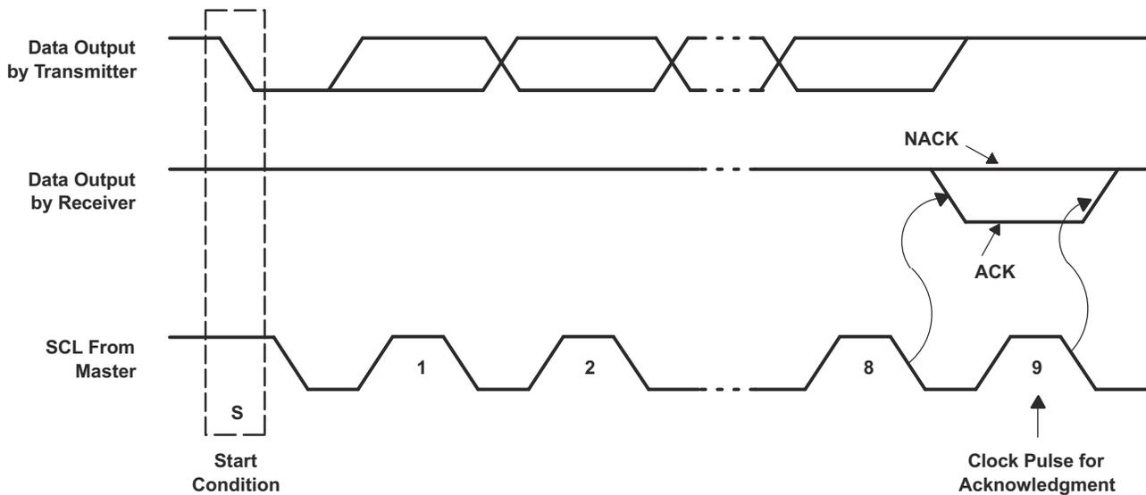
Figure 8-3. Acknowledgment on I<sup>2</sup>C Bus
