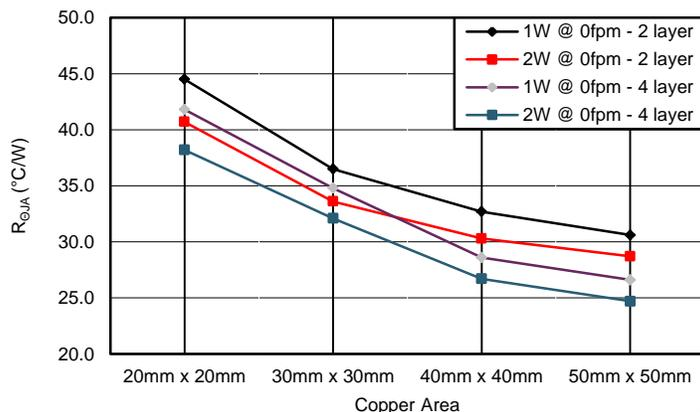
Figure 101. Measured R<sub>θJA</sub> vs PCB Copper Area on a 2-layer Board and a 4-layer Board
