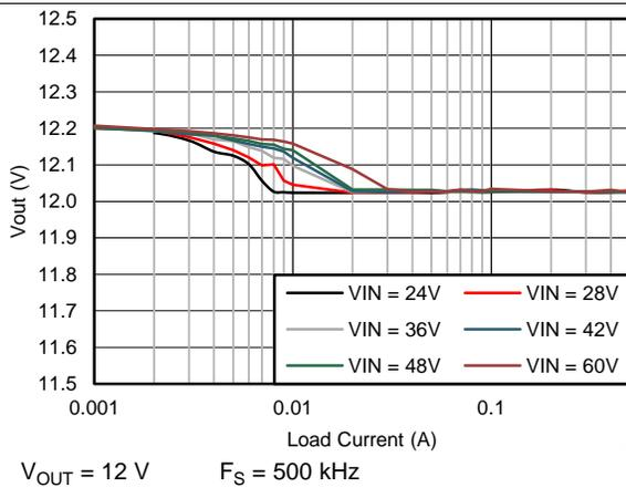
Figure 11.  $V_{OUT}$  Regulation
