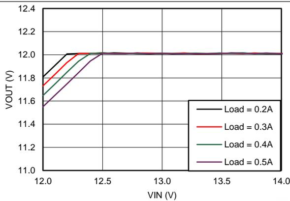
Figure 17. Dropout Curve
