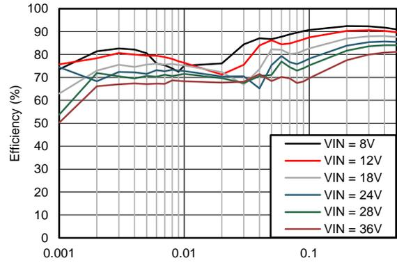
$V_{OUT} = 3.3\text{ V}$   $F_S = 500\text{ kHz}$
