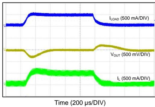
$V_{OUT} = 12\text{ V}$   $F_S = 500\text{ kHz}$   $V_{IN} = 24\text{ V}$
