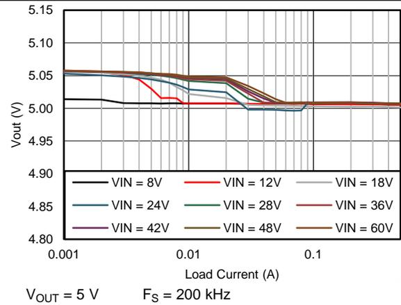
Figure 8.  $V_{OUT}$  Regulation
