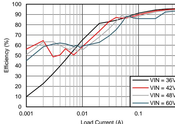
$V_{OUT} = 24\text{ V}$   $F_S = 500\text{ kHz}$
