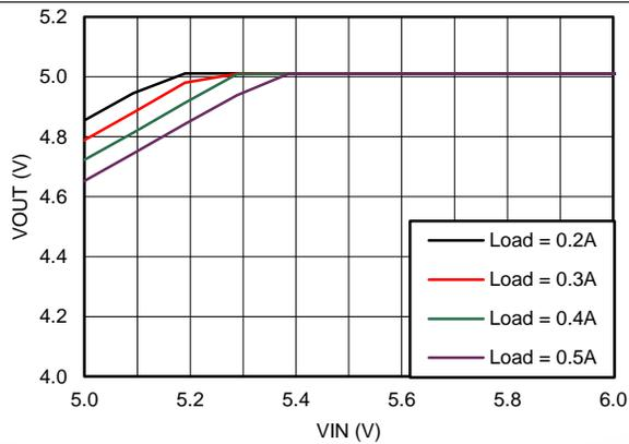
Figure 15. Dropout Curve
