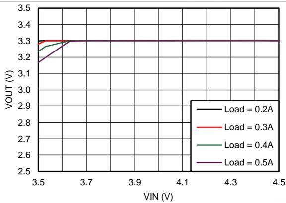
Figure 13. Dropout Curve
