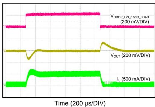
Figure 57. Load Transient Between 0.05 A and 0.5 A
