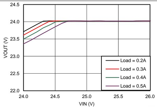
Figure 18. Dropout Curve
