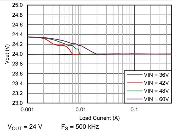
Figure 12.  $V_{OUT}$  Regulation
