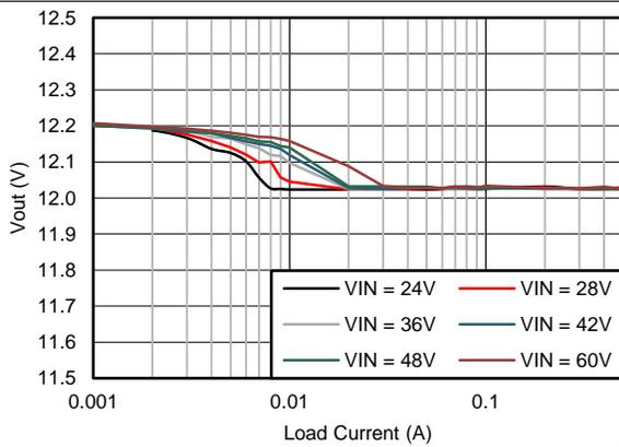
$V_{OUT} = 12\text{ V}$   $F_S = 500\text{ kHz}$
