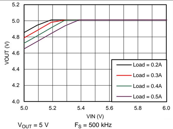
Figure 56. Dropout Curve
