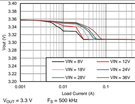
Figure 7.  $V_{OUT}$  Regulation
