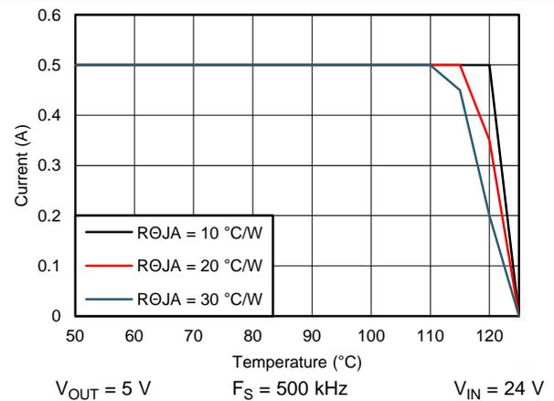
Figure 58. Derating Curve
