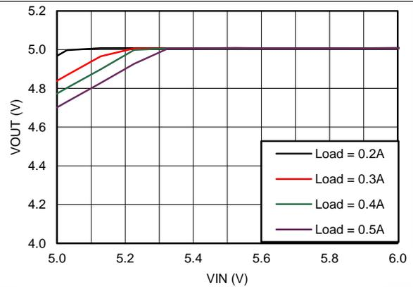
Figure 16. Dropout Curve
