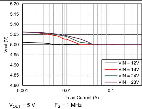
Figure 10.  $V_{OUT}$  Regulation
