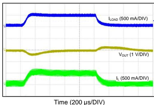
$V_{OUT} = 24\text{ V}$   $F_S = 500\text{ kHz}$   $V_{IN} = 48\text{ V}$
