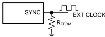
**Figure 41. Frequency Synchronization**
