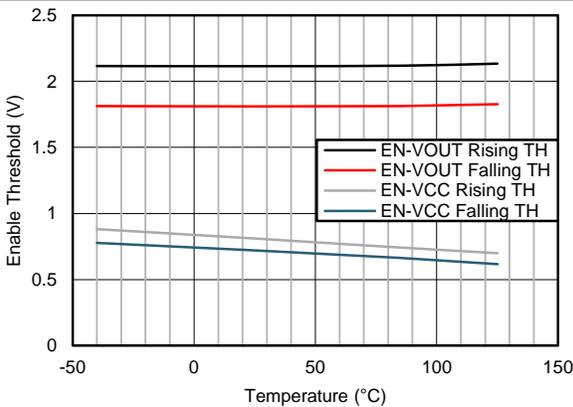
Figure 27. Enable Threshold vs Junction Temperature
