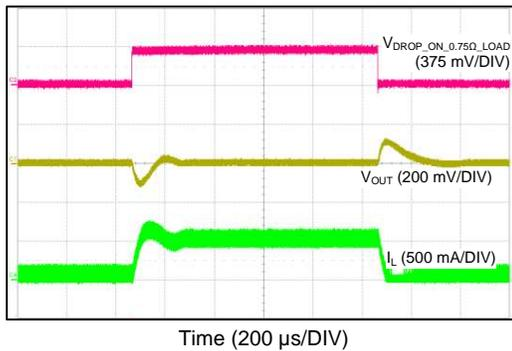
$V_{OUT} = 3.3\text{ V}$   $F_S = 500\text{ kHz}$   $V_{IN} = 24\text{ V}$
