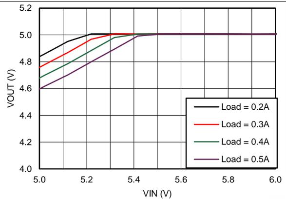
Figure 14. Dropout Curve
