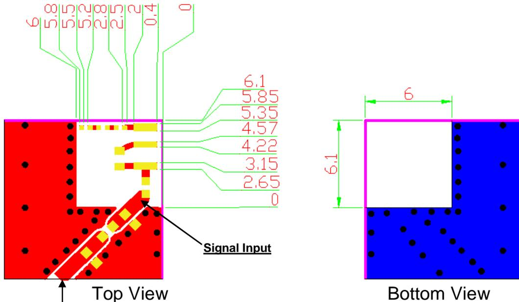
Transmission Line with 50Ω Impedance Characteristic
