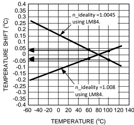
Figure 18. Compensating for an Untargeted Nonideality Factor
