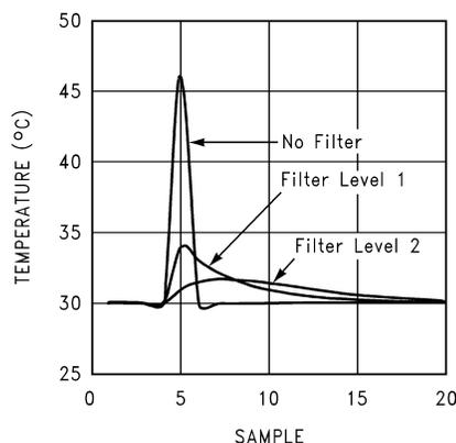
Figure 12. Filter Output Response to a Step Input
