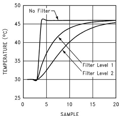
Figure 11. Filter Output Response to a Step Input
