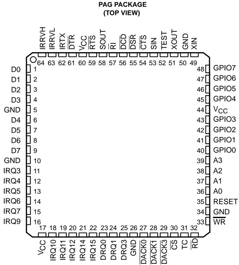
Figure 1–2. Terminal Assignments
