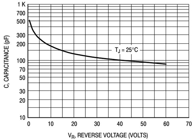
**Figure 6. Typical Capacitance**
