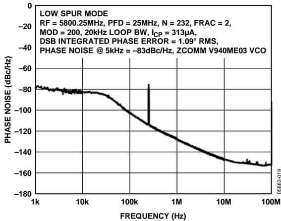
Figure 7. Phase Noise and Spurs, Low Spur Mode
