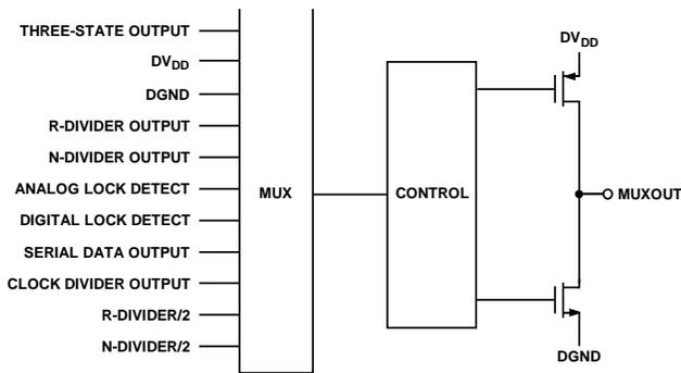
Figure 15. MUXOUT Schematic
