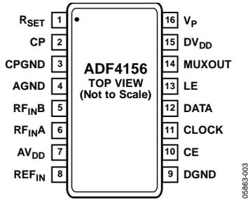
Figure 3. TSSOP Pin Configuration
