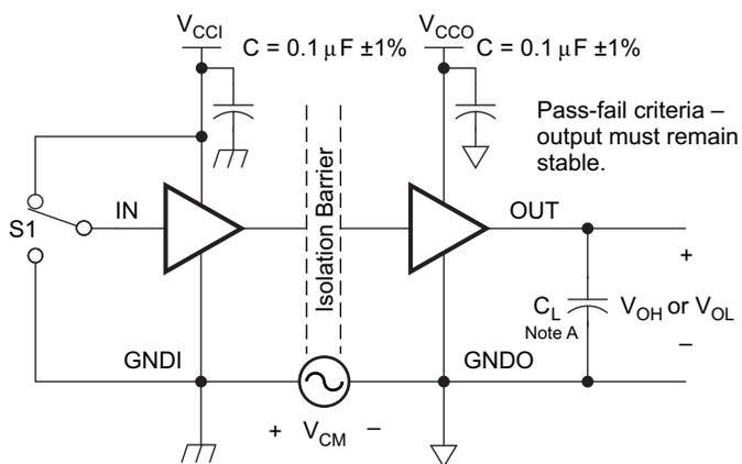
A.  $C_L = 15\text{pF}$  and includes instrumentation and fixture capacitance within  $\pm 20\%$ .
