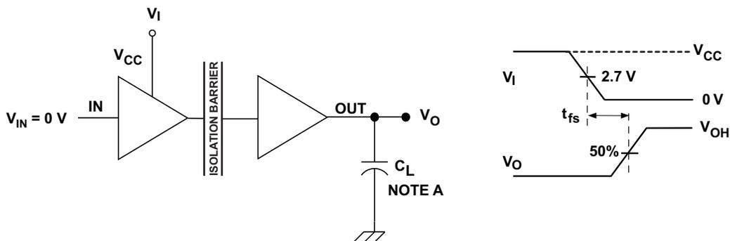
A.  $C_L = 15 \text{ pF}$  and includes instrumentation and fixture capacitance within  $\pm 20\%$ .
