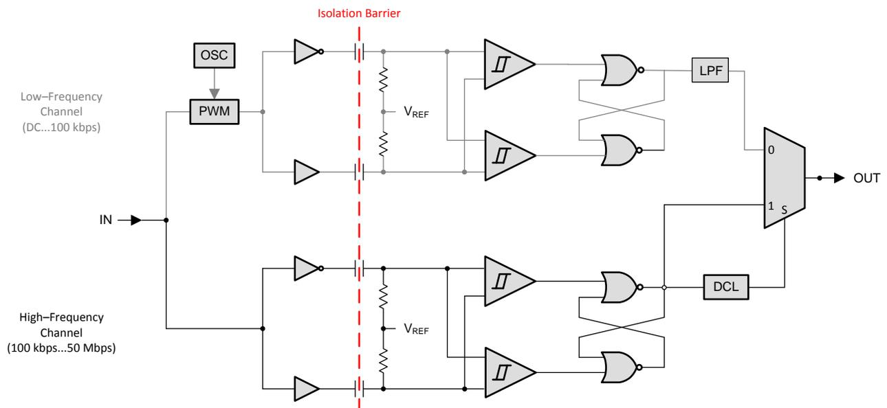
**Figure 12. Conceptual Block Diagram of a Digital Capacitive Isolator**
