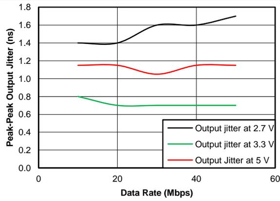
Figure 7. Peak-Peak Output Jitter vs Data Rate
