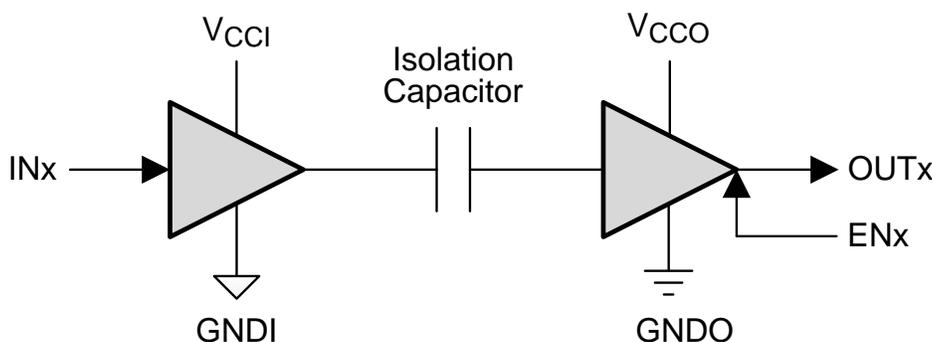
(1) V<sub>CCI</sub> and GNDI are supply and ground connections respectively for the input channels.
