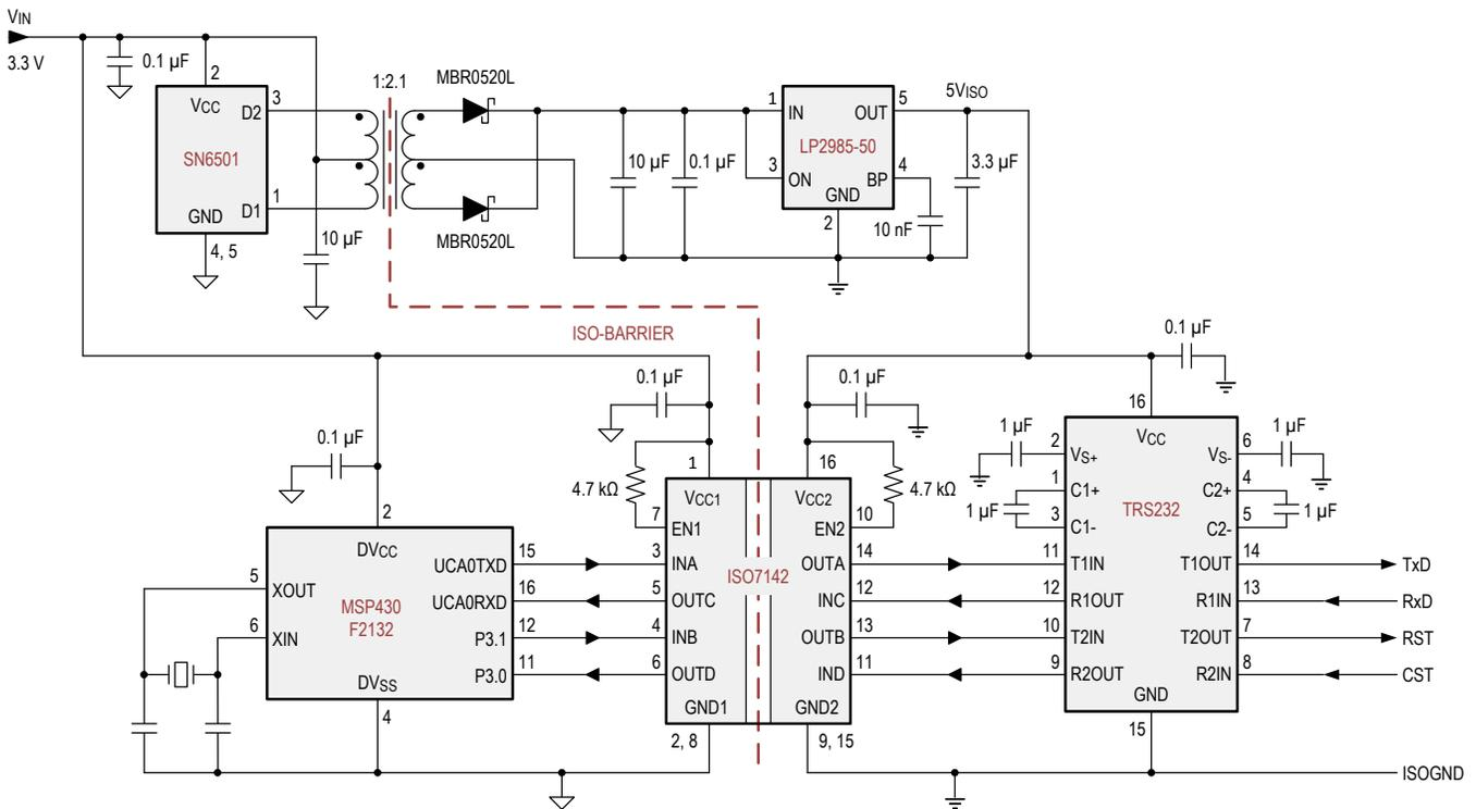
Figure 14. Typical Isolated RS-232 Application Circuit for ISO7142
