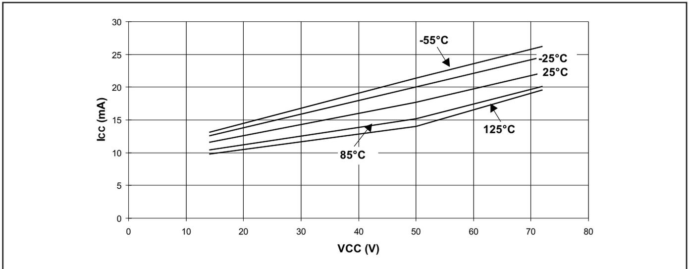
Figure 3. I<sub>CC</sub> vs. V<sub>CC</sub> vs. temperature.
