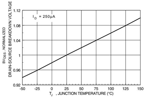
**Figure 7. N-Channel Breakdown Voltage Variation with Temperature.**
