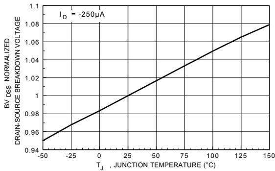
Figure 18. P-Channel Breakdown Voltage Variation with Temperature.
