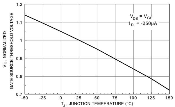
Figure 17. P-Channel Gate Threshold Variation with Temperature.
