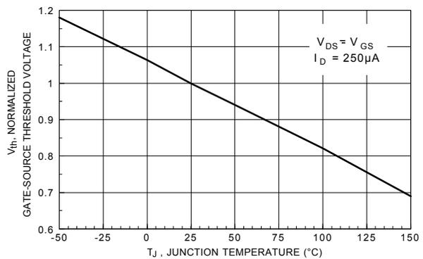
Figure 6. N-Channel Gate Threshold Variation with Temperature.
