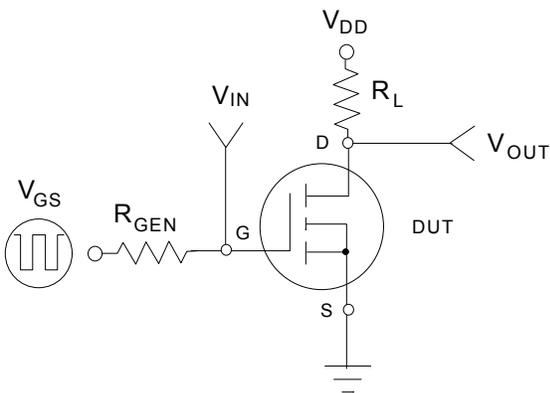
**Figure 29. N or P-Channel Switching Test Circuit.**
