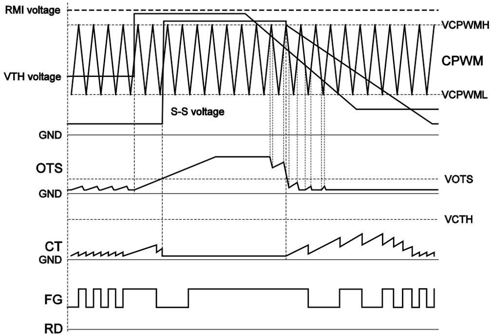
When the output duty ratio based on the VTH/RMI input drops to below 1% or so, the OTS voltage rises, and when it reaches VOTS, the standby mode is established, the CT pin discharges, and the S-S pin is charged. In the standby mode, if the drive mode has been established again by the VTH/RMI input, the rotation is started immediately with soft start. The CT pin discharges at the same time as the switching of FG. For details on lock protection, refer to (2).
