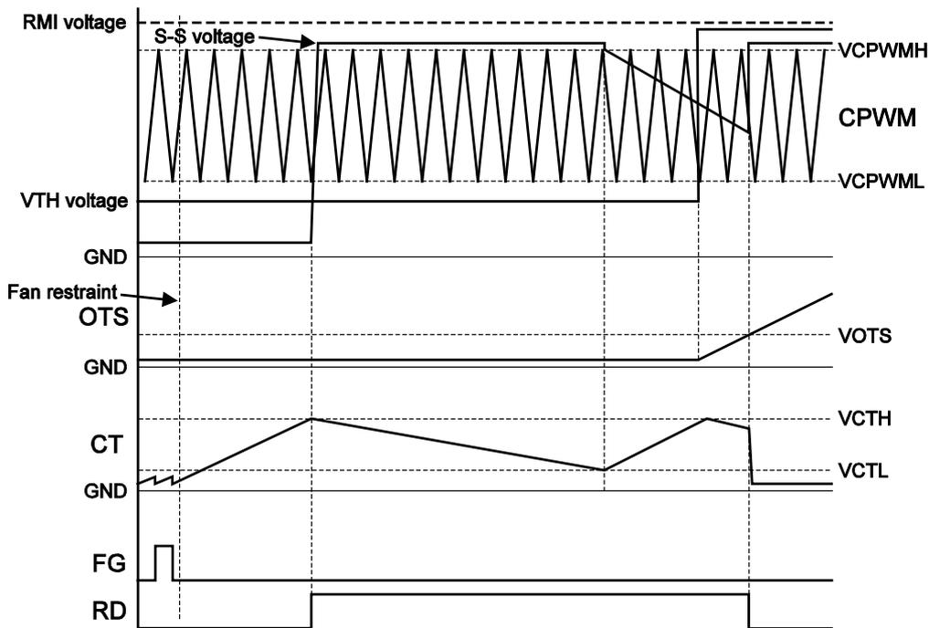
When the fan is constrained, the CT pin voltage rises, and when it reaches VCTH, the lock protection mode is established, and OUTP is set to OFF and RD is set to OFF.
