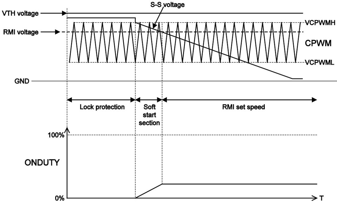
Adjust the S-S pin voltage gradient by means of the capacitance of the capacitor between the S-S pin and REG.
