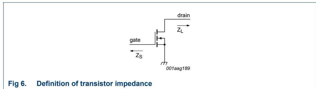
**Fig 6. Definition of transistor impedance**
