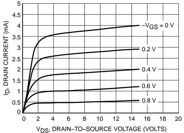
**Figure 3. Drain Current versus
