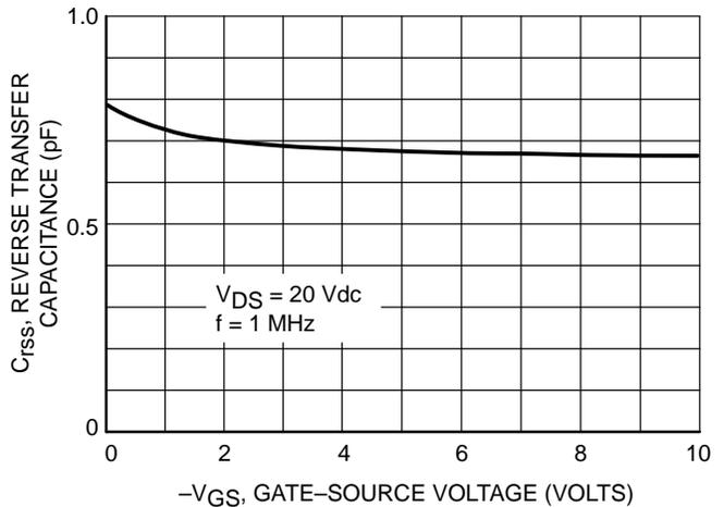
Figure 9. Reverse Transfer Capacitance versus Gate-Source Voltage
