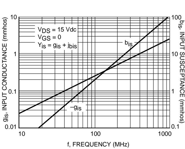
Figure 4. Input Admittance versus Frequency
