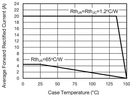
Fig. 1 - Maximum Forward Current Derating Curve
