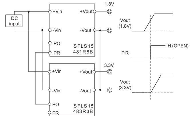
Fig.3.5 PR connection example
