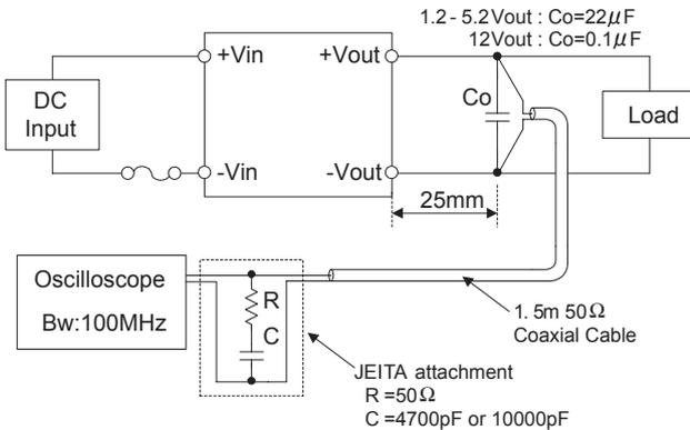
Fig.2.5 Measuring method of ripple and ripple noise
