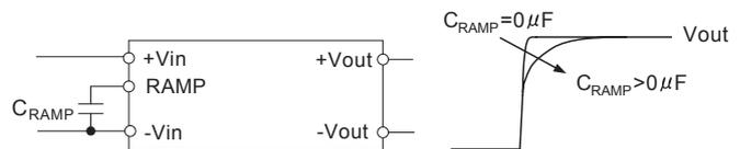
Fig.3.6 Connection method of  $C_{RAMP}$
