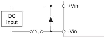
Fig.2.3 Reverse input voltage protection
