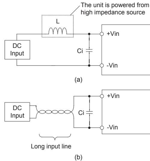
Fig.2.1 Connection method of capacitor at input pin
