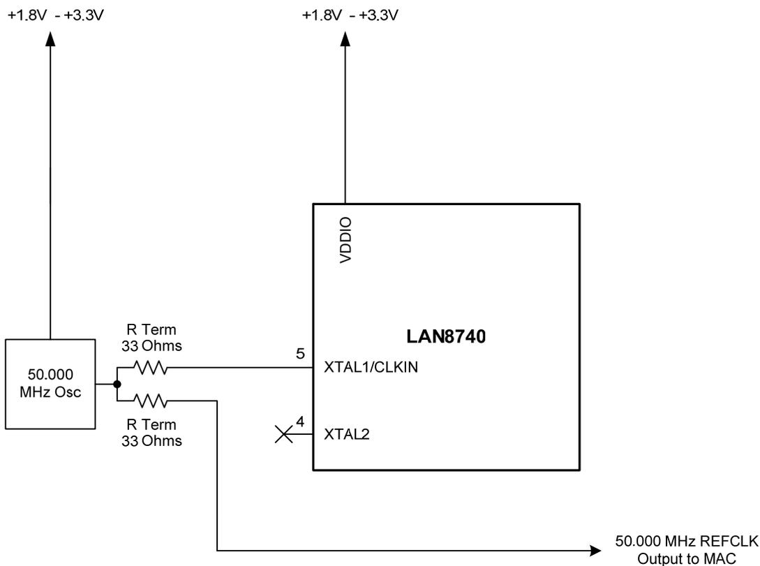
Figure 5 – LAN8740 Clock Oscillator Connections
