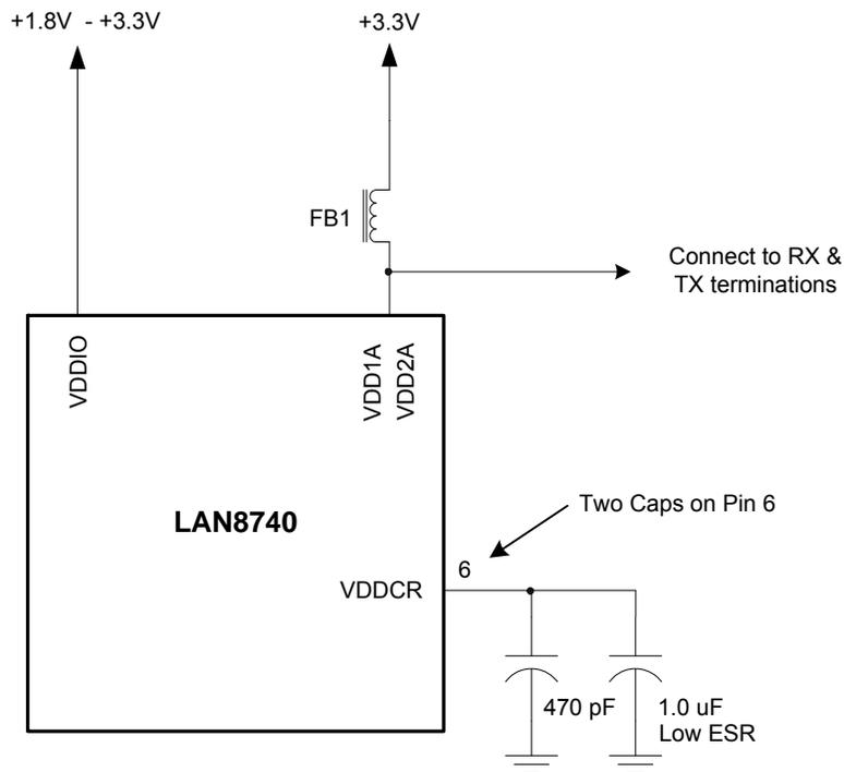
Figure 3 - LAN8740 Power Connections
