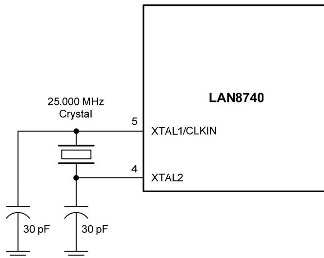
Figure 4 – LAN8740 Crystal Connections
