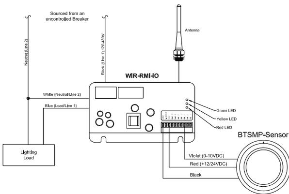
NOTE: Disconnect power prior to installation.
