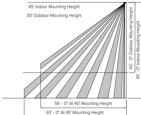
Sensor Lens Coverage and Detection Patterns
