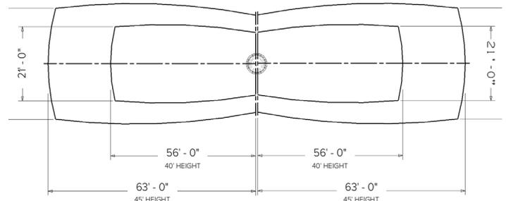
Sensor Lens Coverage and Detection Patterns
