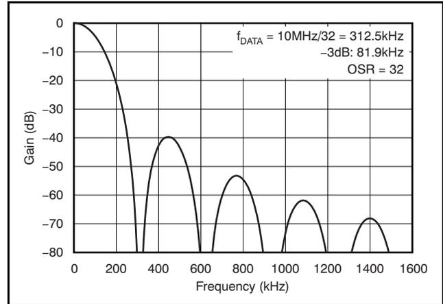
Figure 25. Frequency Response of the Sinc<sup>3</sup> Filter
