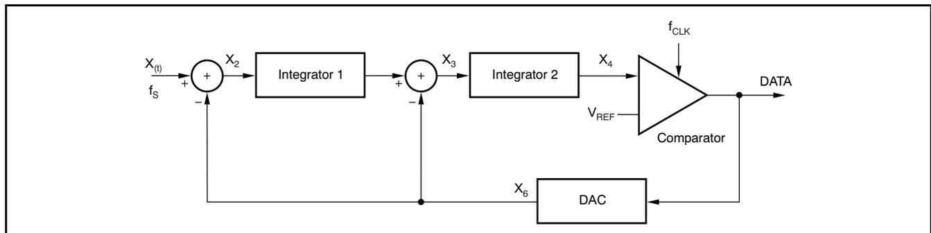
**Figure 24. Block Diagram of the 2nd-Order Modulator**
