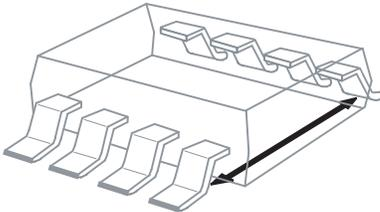
**Input-to Output Barrier Capacitance:** The total capacitance between all input terminals connected together, and all output terminals connected together.
