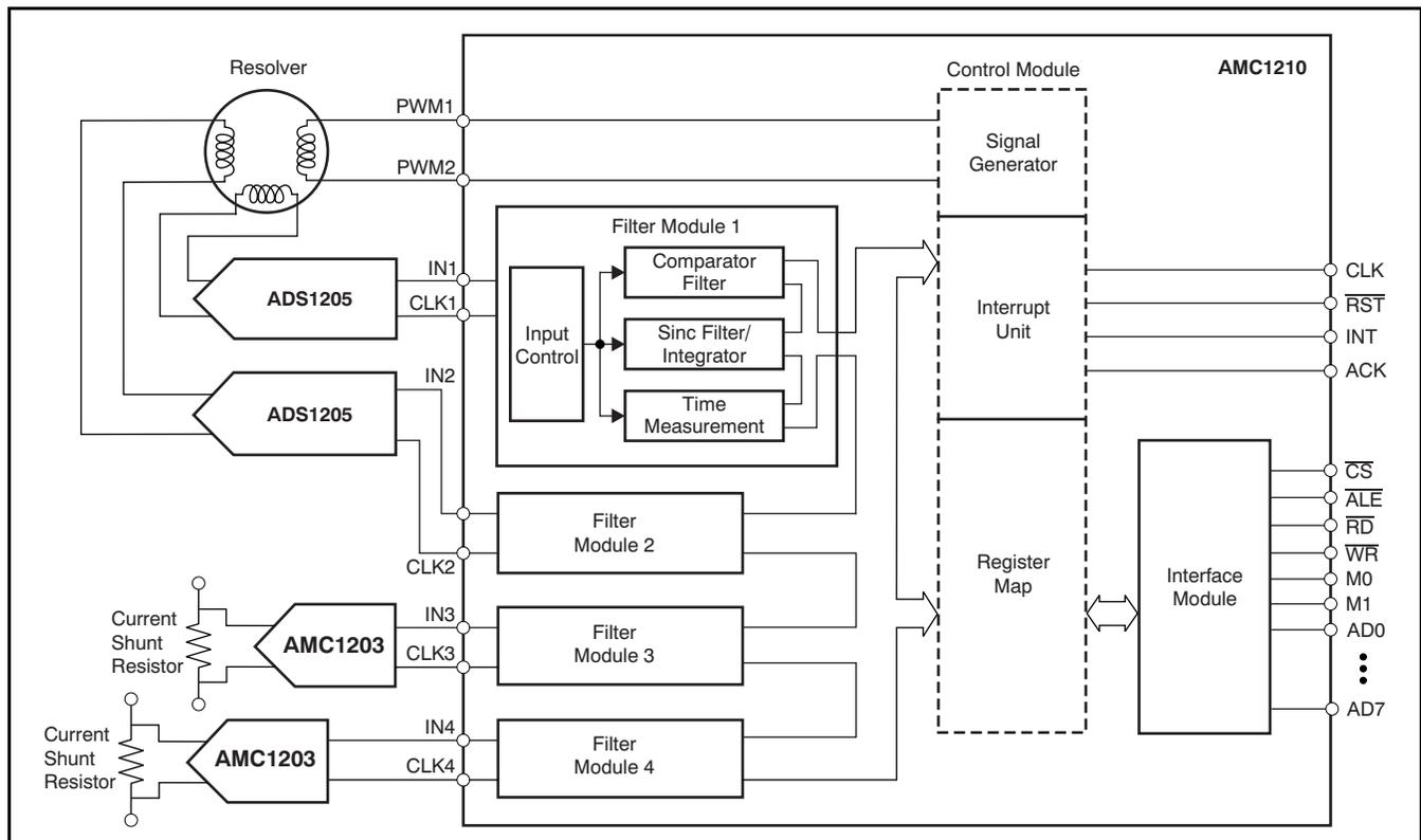
Figure 23. Example of a Resolver-Based Motor-Control Application
