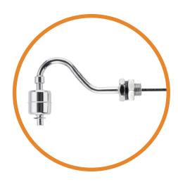
This switch is designed to give the switch level accuracy of a vertical switch, but without the need to mount the switch in the top of the tank. This can also avoid the need for a long vertical top mounted switch, as this switch can be mounted at the required level in the side of the tank.
