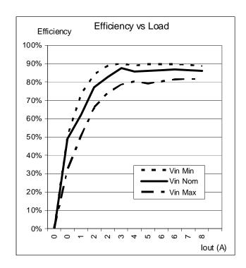
$<sup>^2</sup>$  Measured with a 1  $\mu\text{F}$  ceramic capacitor across output pins, as shown on page 9
