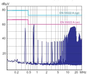
To meet level B, it is necessary to fit a 5  $\mu F$  ceramic capacitor across the input terminals.
