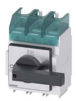
SENTRON, switch disconnector 3LD, main switch, 3-pole, lu: 160 A, operating performance / at AC-23 A at 400 V: 75 kW, installation in distribution boards, knob-operated mechanism, black, handle direct at the switch
