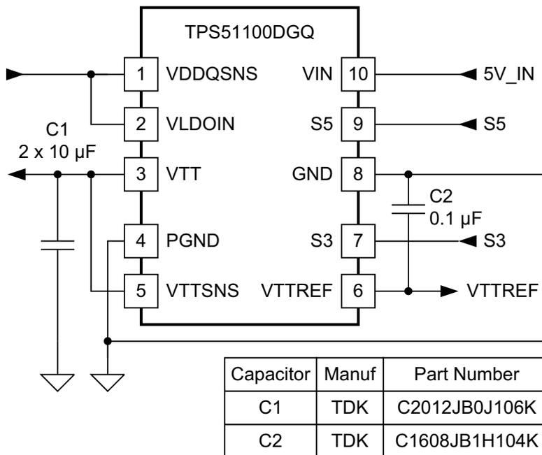
Figure 23. TPS51100 5-V Input / 1.8-V Output Reference Design
