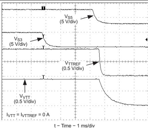
Figure 17. Shutdown Waveforms S3 and S5 High-to-Low
