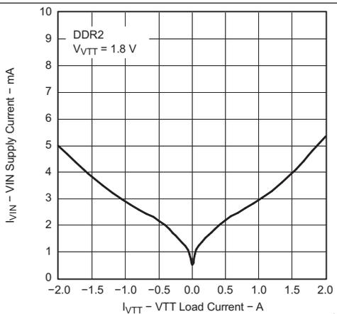
Figure 3. VIN Supply Current vs VTT Load Current
