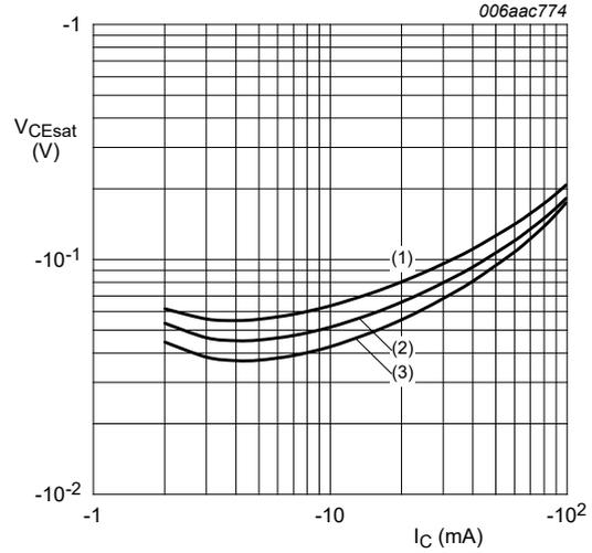
Fig. 12. TR2 (PNP): Collector-emitter saturation voltage as a function of collector current; typical values
