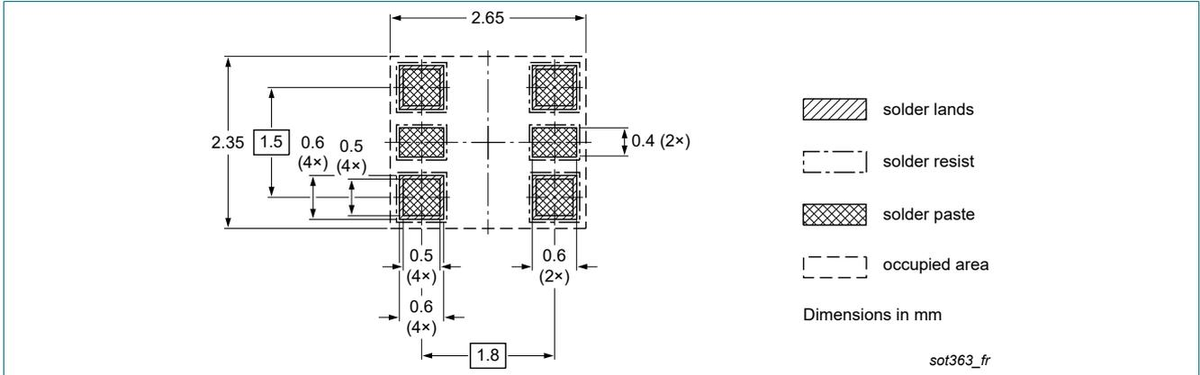
Fig. 20. Reflow soldering footprint for TSSOP6 (SOT363)
