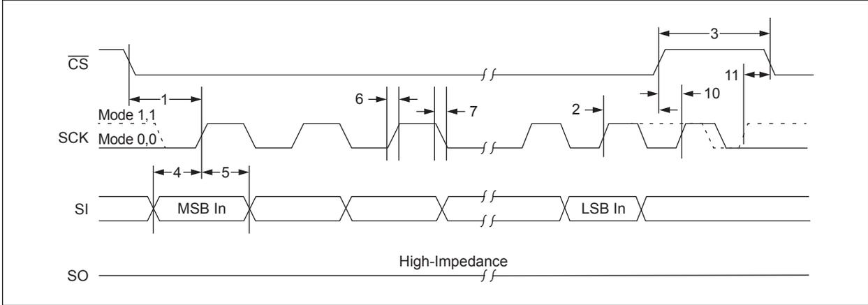
FIGURE 12-11: SPI OUTPUT TIMING
