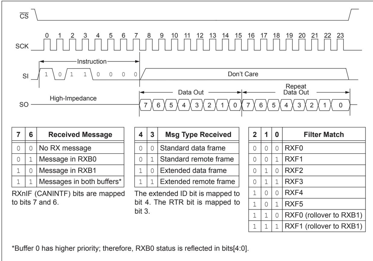
FIGURE 12-10: SPI INPUT TIMING
