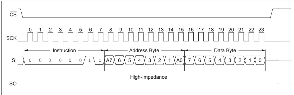
**FIGURE 12-5: LOAD TX BUFFER INSTRUCTION**
