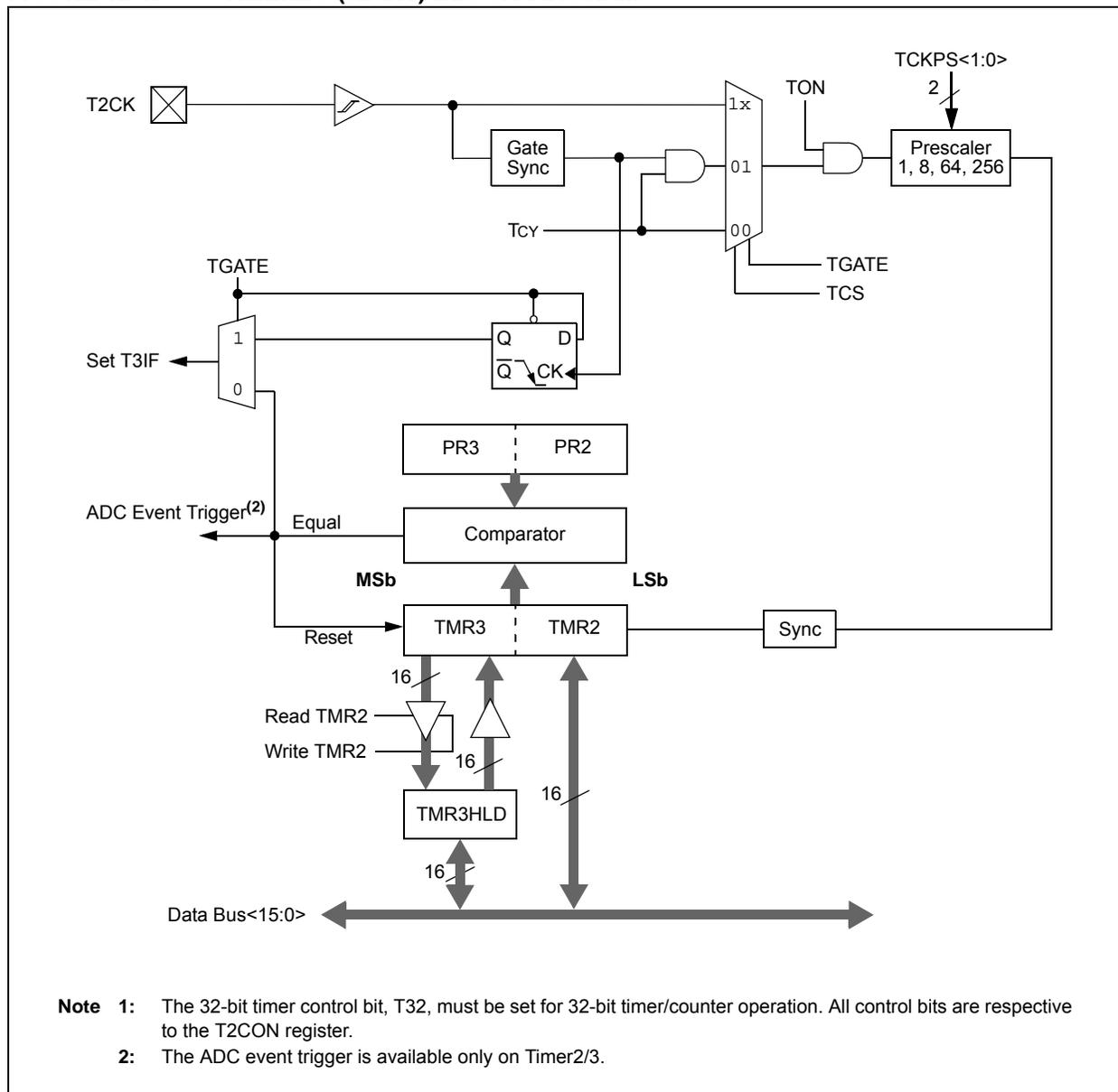
**FIGURE 12-2: TIMER2 (16-BIT) BLOCK DIAGRAM**
