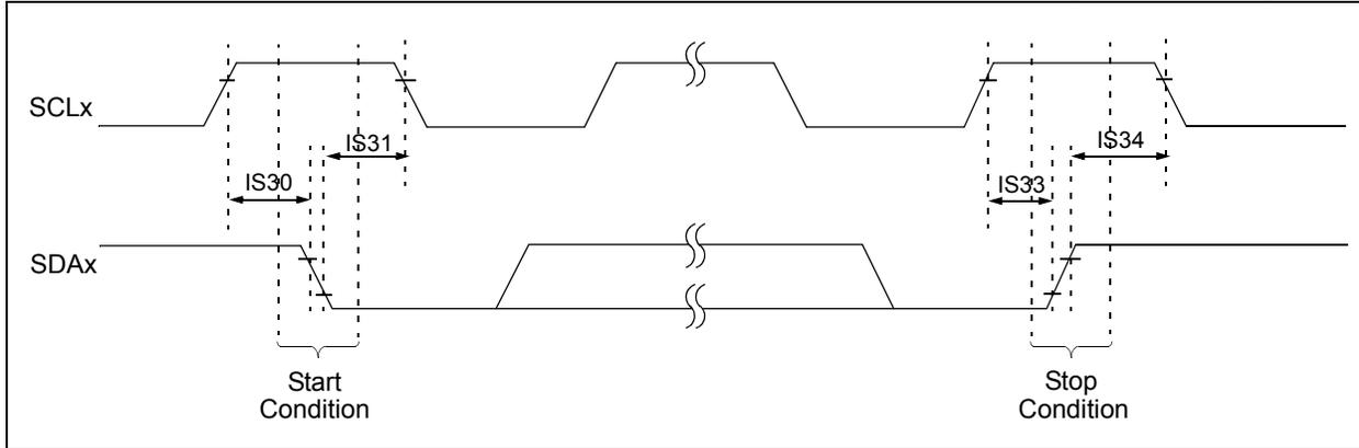
**FIGURE 24-25: I2Cx BUS DATA TIMING CHARACTERISTICS (SLAVE MODE)**
