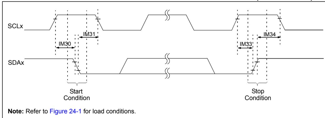
**FIGURE 24-23: I2Cx BUS DATA TIMING CHARACTERISTICS (MASTER MODE)**
