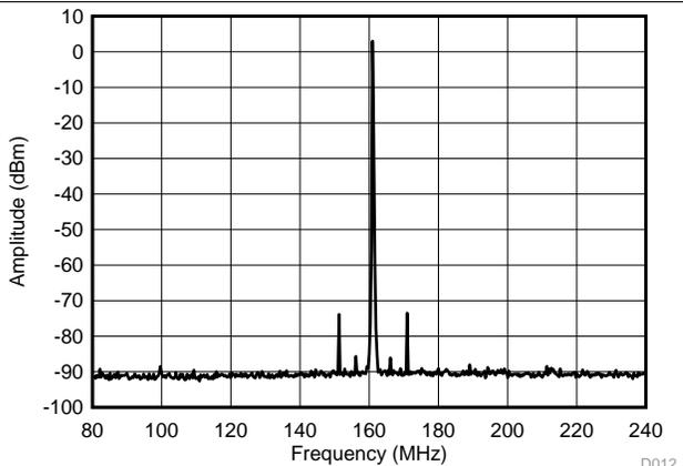
PLL Bandwidth = 400 kHz      VCO Frequency = 5.15625 GHz
