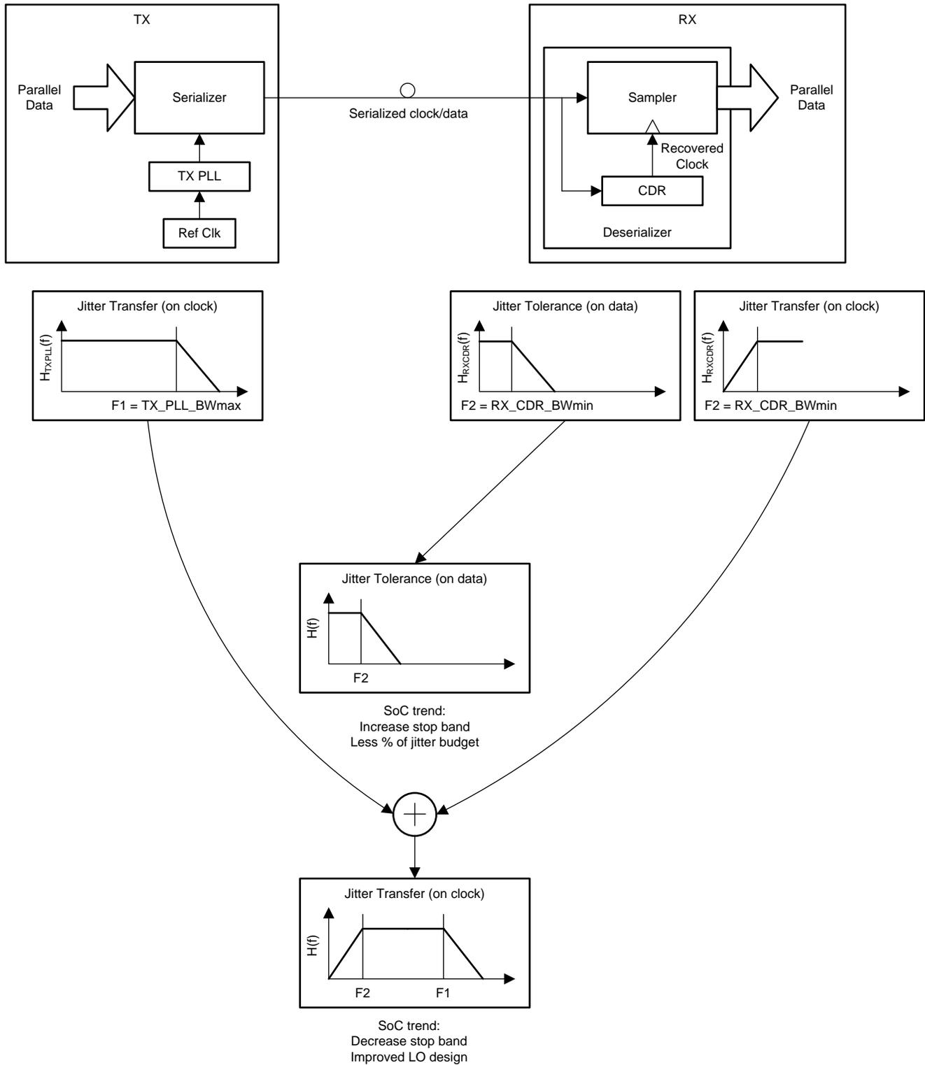
Figure 32. Dependence of Clock Jitter in Serial Links
