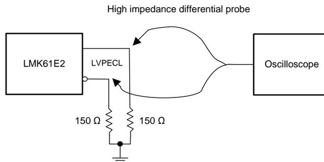
Figure 16. LVPECL Output DC Configuration During Device Test
