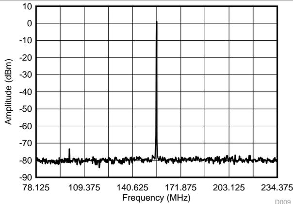
PLL Bandwidth = 400 kHz      VCO Frequency = 5 GHz
