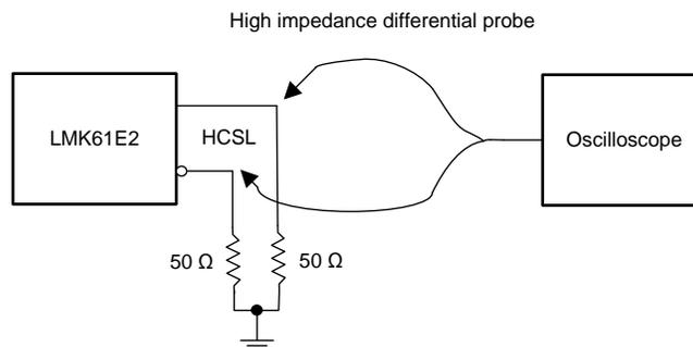
Figure 18. HCSL Output DC Configuration During Device Test
