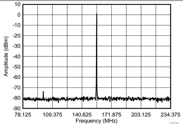
PLL Bandwidth = 400 kHz      VCO Frequency = 5 GHz
