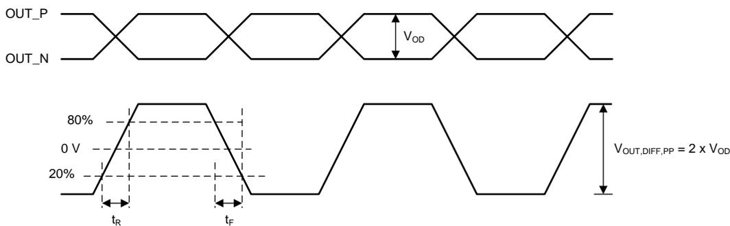
Figure 23. Differential Output Voltage and Rise/Fall Time
