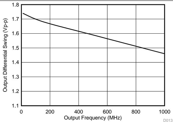
**Figure 13. LVPECL Differential Output Swing vs Frequency**
