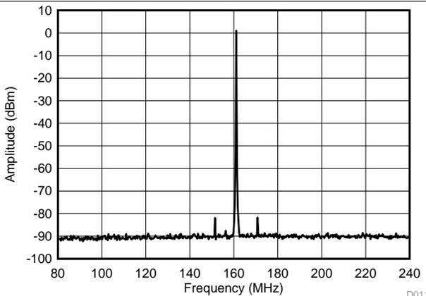
PLL Bandwidth = 400 kHz      VCO Frequency = 5.15625 GHz
