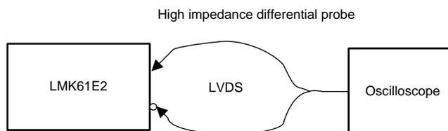
Figure 17. LVDS Output DC Configuration During Device Test
