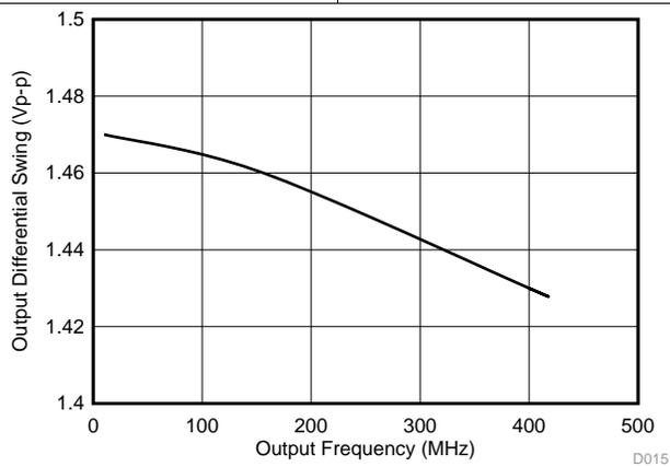
**Figure 15. HCSL Differential Output Swing vs Frequency**
