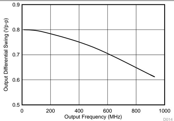
**Figure 14. LVDS Differential Output Swing vs Frequency**
