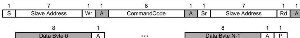
Figure 31. Block Register Read Programming Sequence
