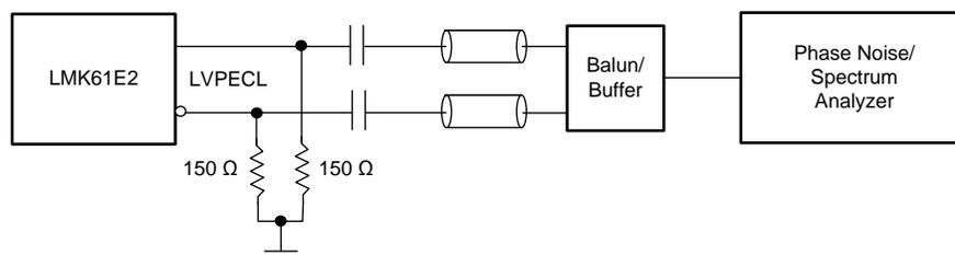
Figure 19. LVPECL Output AC Configuration During Device Test
