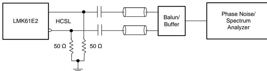
Figure 21. HCSL Output AC Configuration During Device Test
