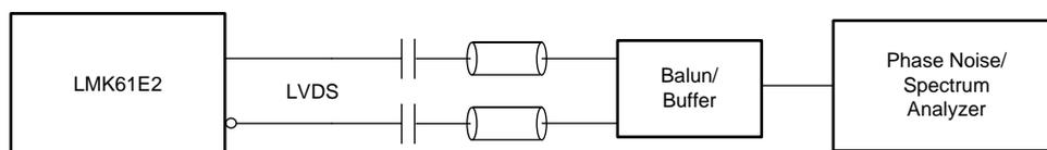
Figure 20. LVDS Output AC Configuration During Device Test
