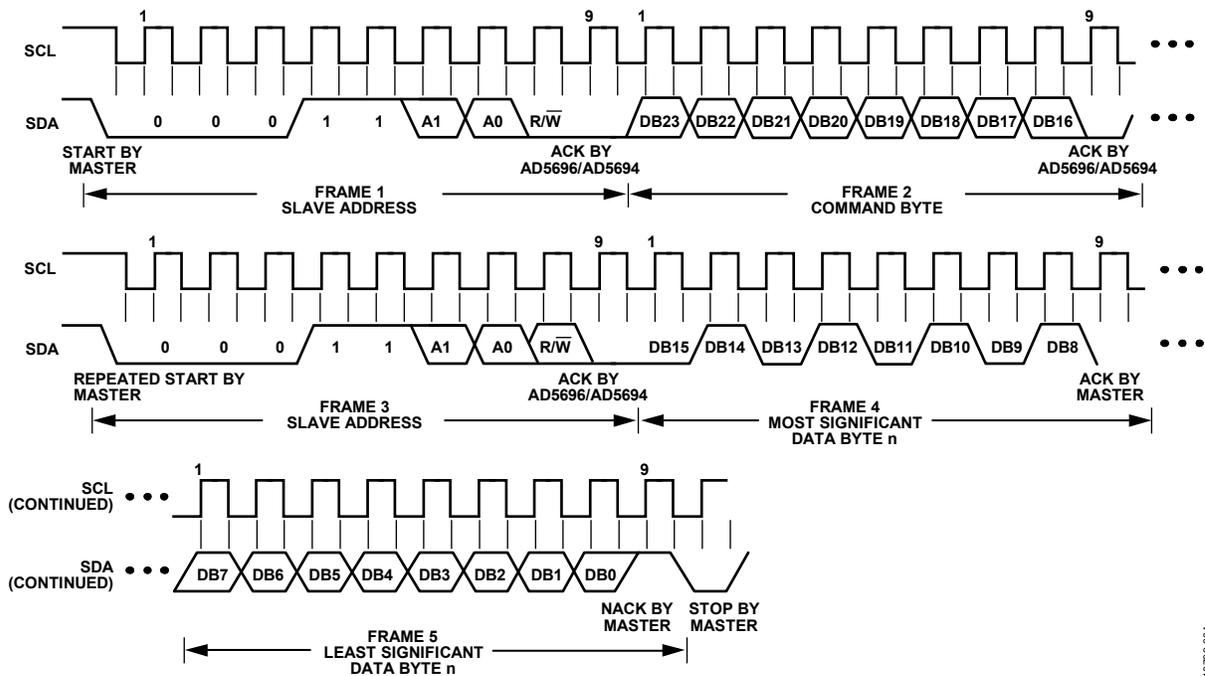
Figure 38. I<sup>2</sup>C Read Operation
