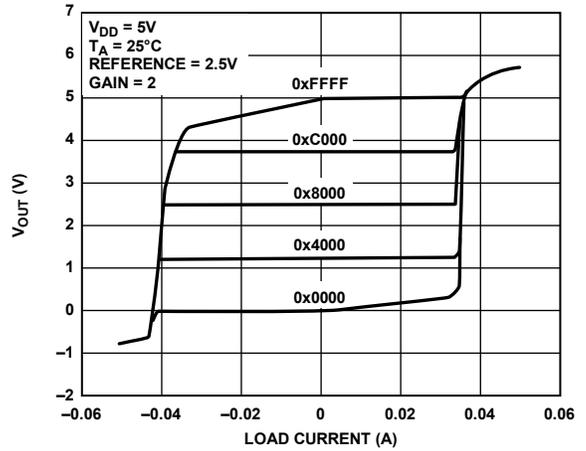
Figure 21. Source and Sink Capability at 5 V
