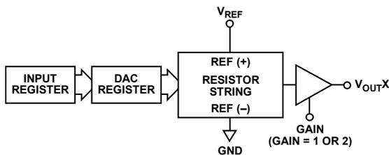
Figure 33. Single DAC Channel Architecture Block Diagram
