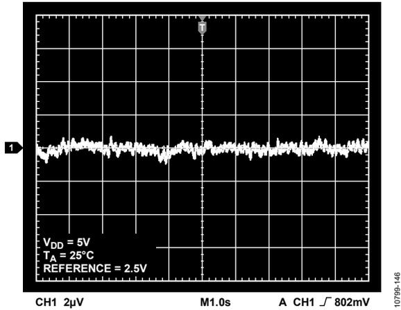
Figure 29. 0.1 Hz to 10 Hz Output Noise Plot
