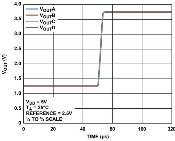
Figure 24. Settling Time
