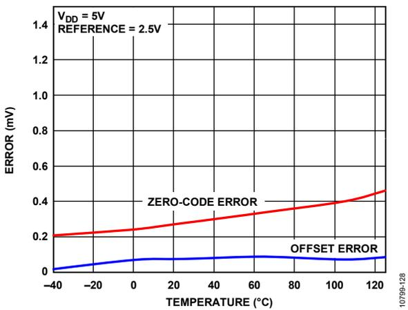
Figure 13. Zero-Code Error and Offset Error vs. Temperature
