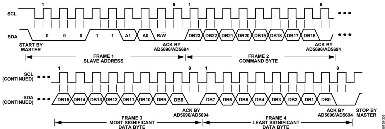
Figure 37. I<sup>2</sup>C Write Operation
