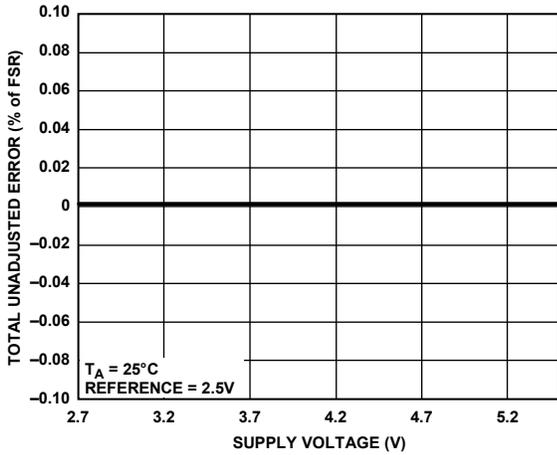
Figure 17. TUE vs. Supply Voltage, Gain = 1
