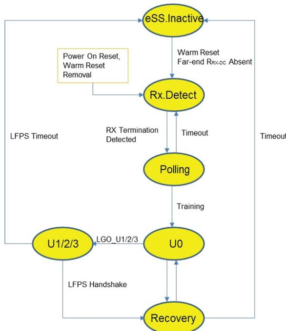
**Figure 4-3 Re-timer Supported USB Power State Diagram**
