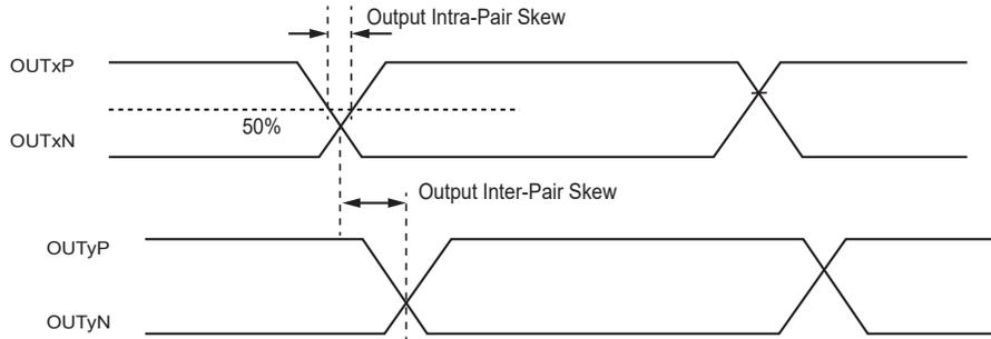
**Figure 5-2 Intra and Inter-pair Differential Skew Definition**
