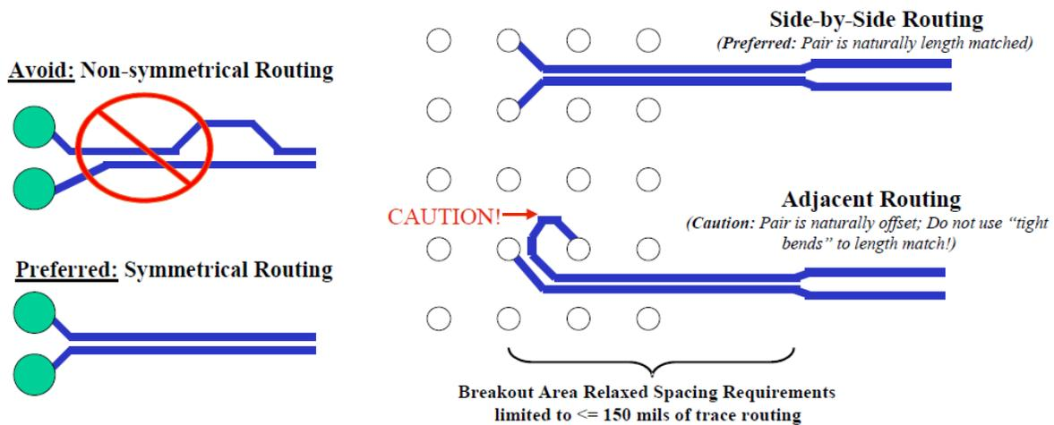
**Figure 6-7** Layout Guidance of Matched Differential Pair
