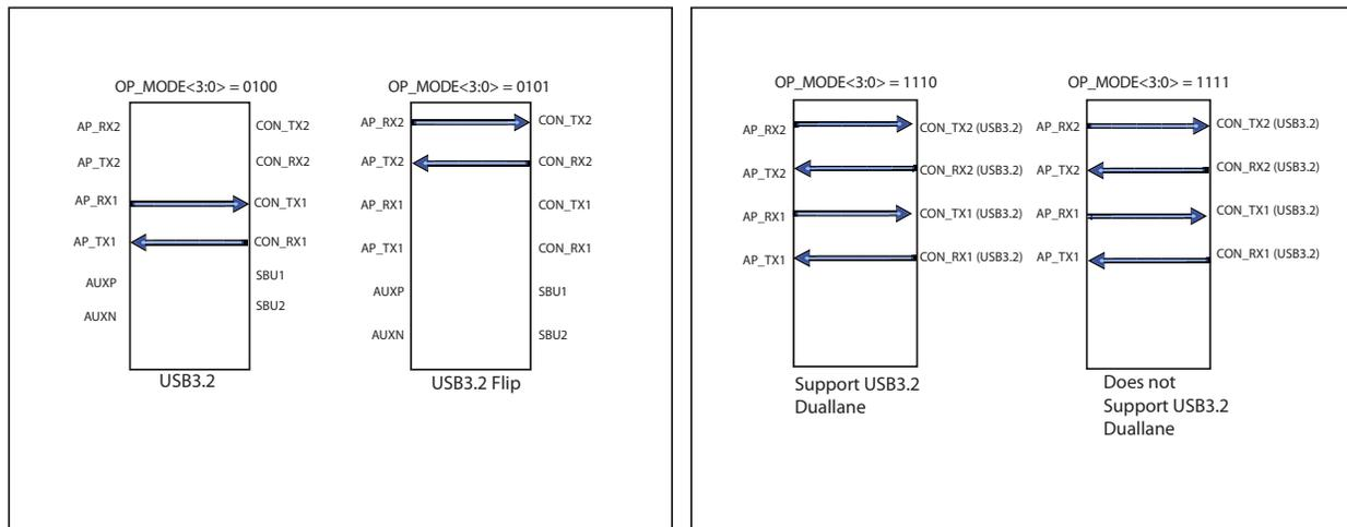
**Figure 2-1 The Channel Configuration Against the  $OP\_MODE\langle 3:0 \rangle$**
