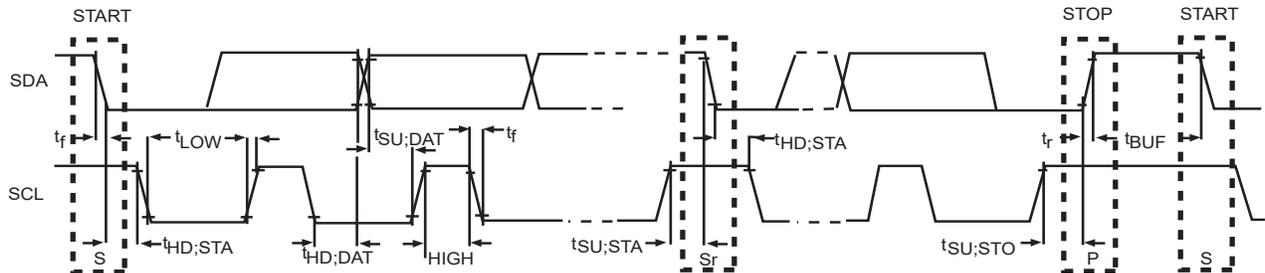
**Figure 5-4 Definition of Timing on the I2C-Bus**
