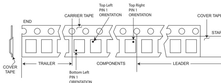
**Figure 7-4 Tape Leader and Trailer Pin 1 Orientations**
